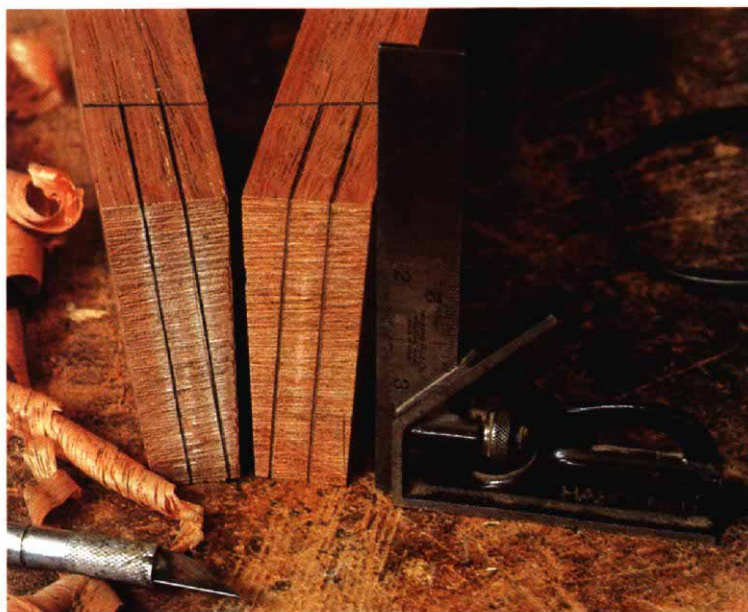
Top, the reflection on the side seat rail highlights the strategy for 'twisting' it to meet the splayed rear post—the surface is planed down along the diagonal. In normal lighting, the rail looks flat, with the twist more easily felt than seen. Lower photo shows the rear tenons on the rails (scribed marks darkened for clarity).
