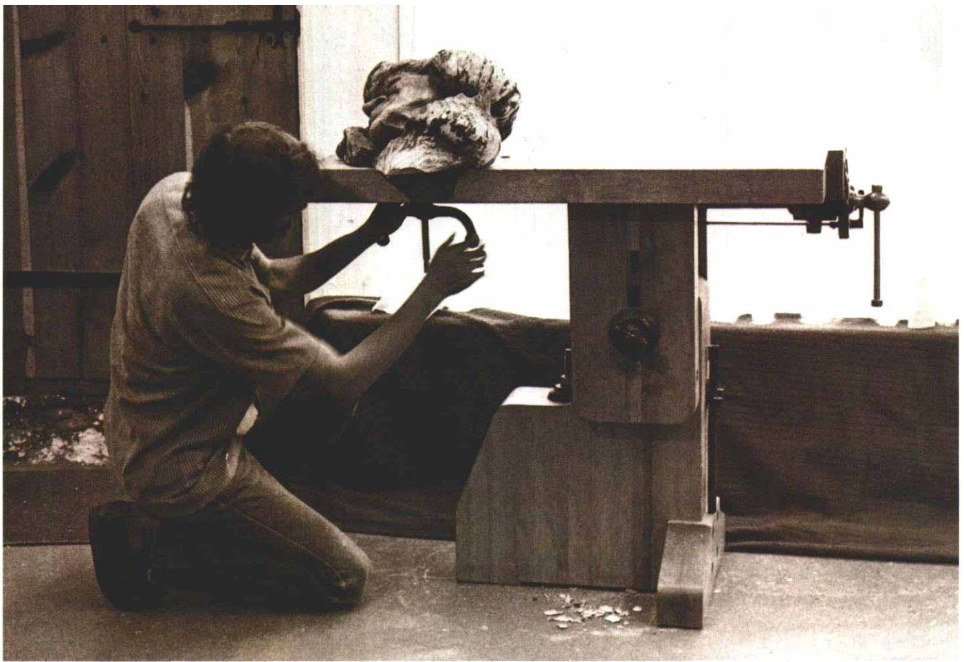
Cloutier secures the carving with a carvers' screw, above, then tips the bench, raising the piece to a comfortable work height, below.
