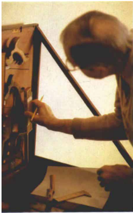
Lynch prefers a folding carpenter's rule, left, because it won't snap back as a steel tape might. Holding his bevel gauge handle parallel to the chest corner, he angles its tongue to match the dovetails, above. He records the angle with a protractor. For something as irregular as this tavern table leg, he uses a simple pen holder to trace contours. The Plexiglas edge of the wooden upright is set directly over the angled pen. As you run the plastic along the piece, the pen records the contour on paper on the instrument's base.
