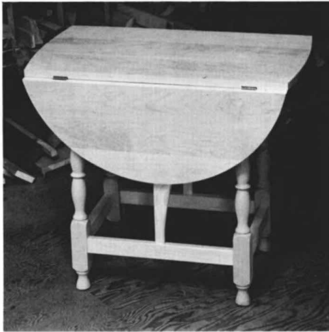
Cohasset Colonial's standard butterfly table has upright legs and a butt leaf-joint. The author's version, which incorporates a few modifications, is shown in the photo on p. 76.
