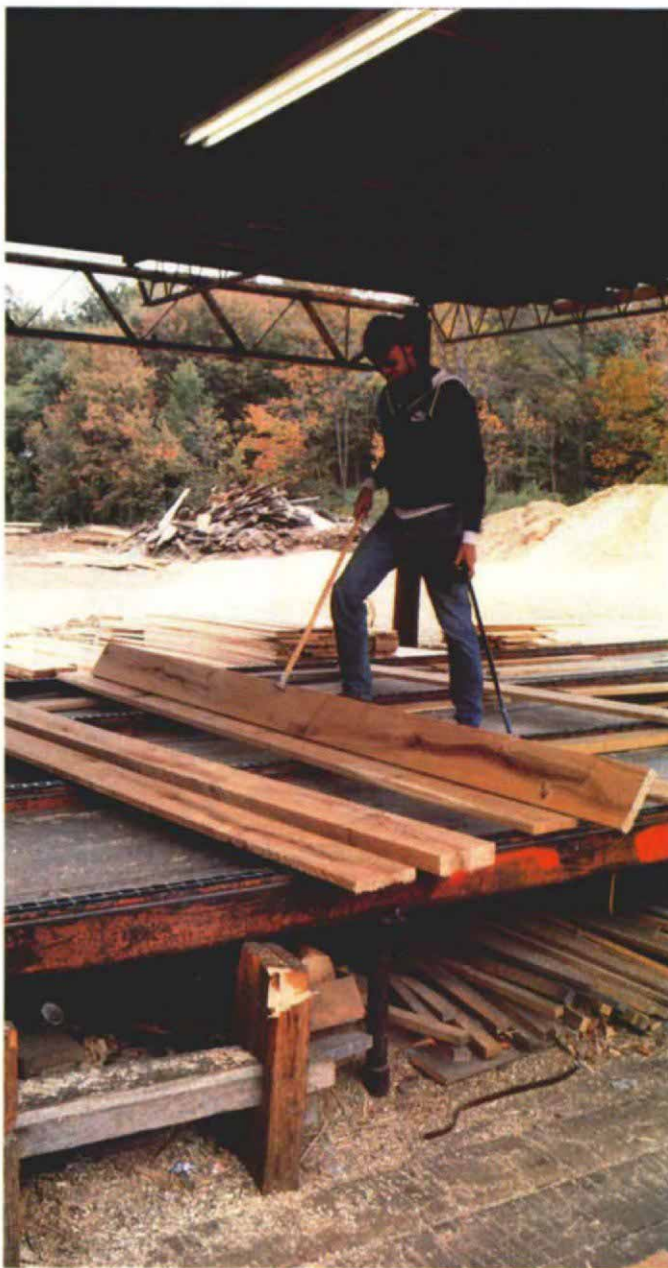
To choose the grading face, grader Wally Cole flips a red-oak board with his steel-tipped lumber rule. Cole marks a grade with his crayon-tipped wand and records the surface measure and grade in the logbook in his left hand.
