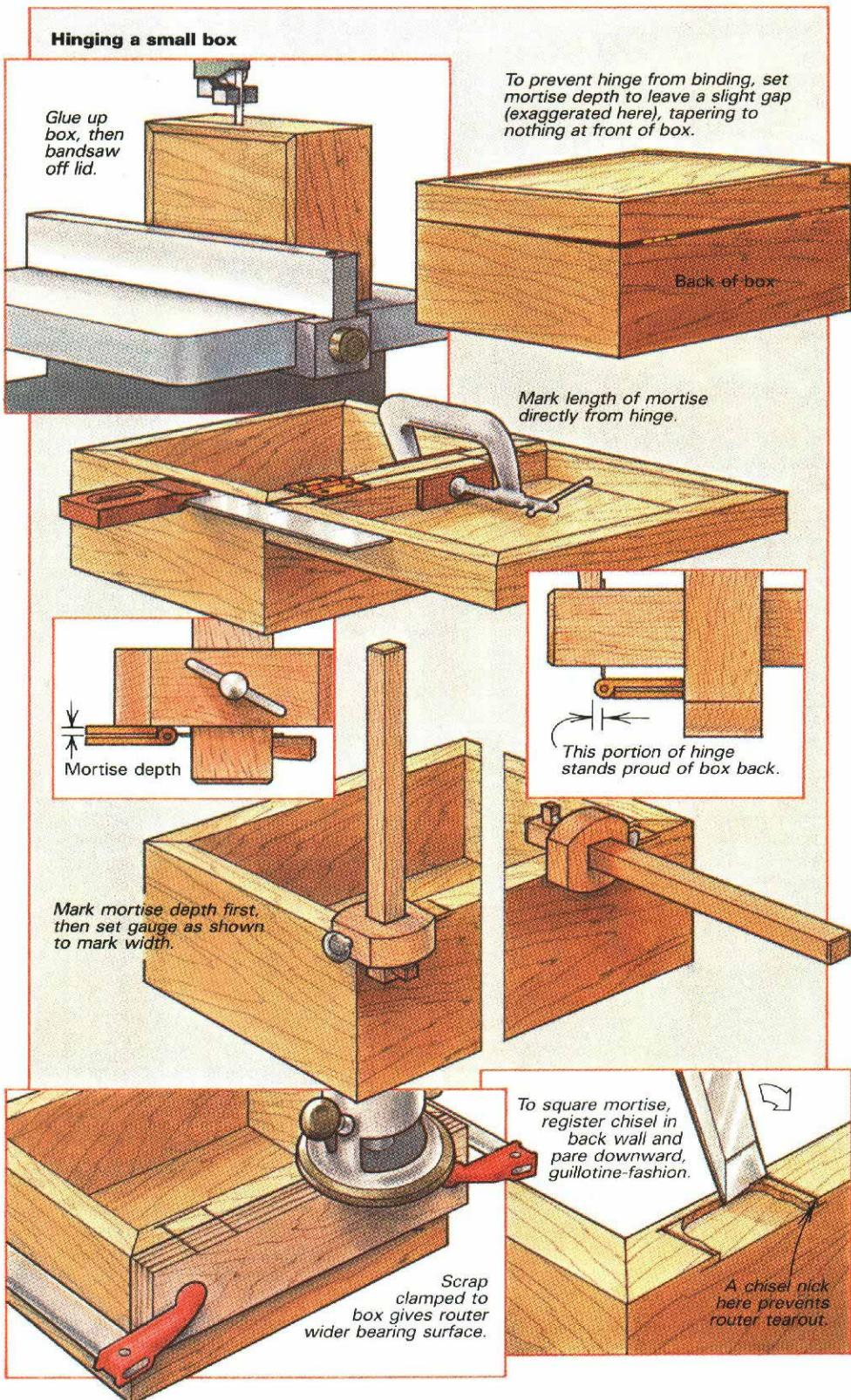
depth. Single or double, it's the barrel, not the leaf thickness, that governs depth. I make the mortise a touch shallow, which leaves a tiny gap at the back of the box but ensures that the front will close nicely.
