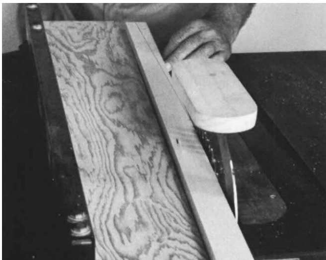
Ripping the taper: Jig guarantees four identical slides.
