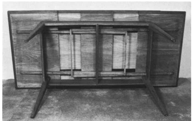
Partly open view from below shows system of slides, stops.
