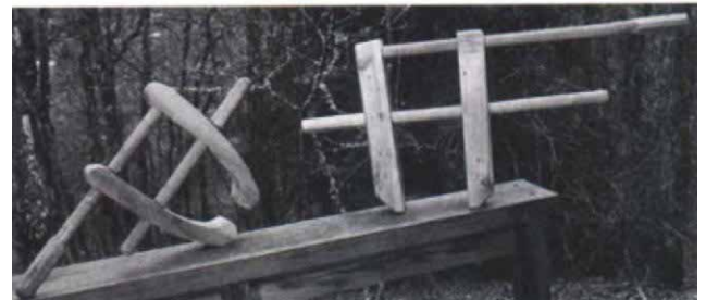
Wooden hand screws may be made in almost any size, with jaws and handles shaped to fit particular types of work.
