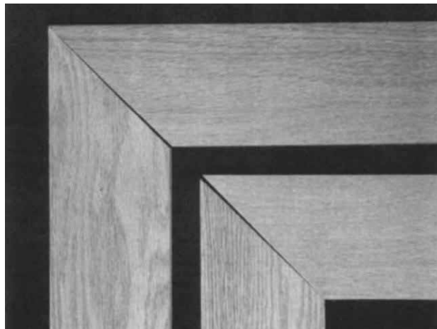
These two red oak frame corners were tightly mitered when originally assembled. The upper one was dried, the lower one dampened. Since wood is stable along the grain, but shrinks and swells across the grain, joints open as shown.
