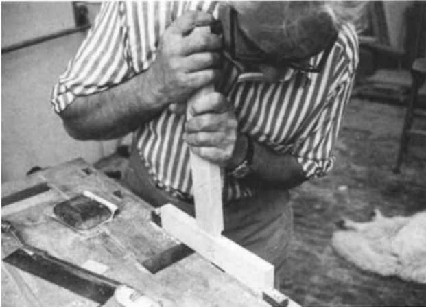
cheeks because that's the easier piece to correct. If the tenon is too loose, you can glue strips of veneer to the cheeks.
