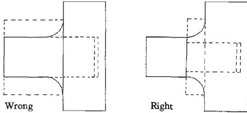
prevent problems with the end grain which will break and crumble, especially if carved.
