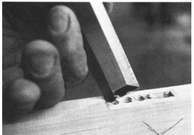
mortise piece as you did the tenon sides and you're ready to try the fit. You should be able to push it in by hand with the weight of your body. If you need to hammer it in, it's too tight and you should shave some material off the tenon
