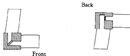
Usually the angle is made in the tenon, because it is easier than angling the mortise. Of course there is a limit to how much the tenon can be angled, but as long as some long grain reaches the full length of the tenon, it is safe.
