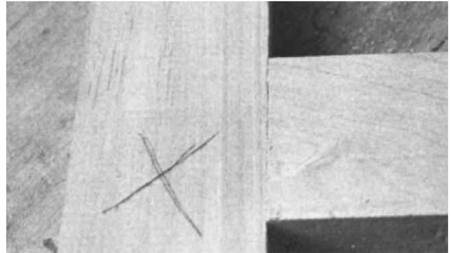
On complicated pieces where the joints may come in at odd angles, I sometimes don't worry about precise fitting of the shoulders during the initial cutting process, but rely instead on the correction cuts to get the fit I want.
