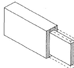
four shoulders must be precisely located in the same plane. Also, glue surface is lost. On the other hand, if the design calls for carving and material will be removed around the joint, four shoulders ensure that the joint will not be revealed.
