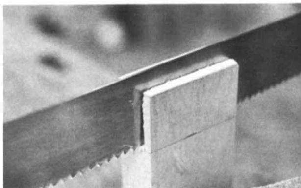
guided at the back by the kerf you made before. You'll also get a little more accuracy in this guiding process if you use a slightly thinner blade for cutting the back lines than you do for cutting the front.
