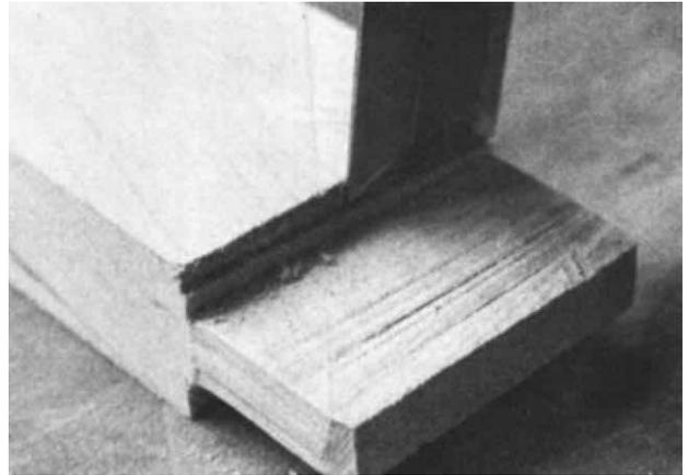
the shoulders is off after you've dry clamped it, make the shoulder correction cuts to all the shoulders on the same side of the frame, so that after correction, the frame stays square (but one blade width shorter). Of course, if a shoulder is really off, you may need to go through the correction process twice.
