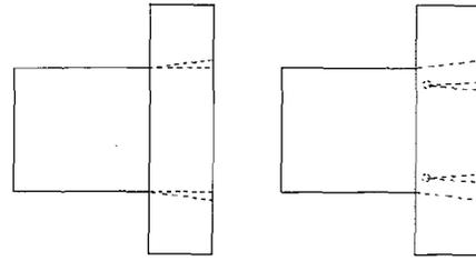
base of the saw cut to prevent cracking. When hammering in wedges in a through tenon, be sure to hammer evenly on each wedge so as not to force one half or the other too far which could result in splitting. If the tenon is to be hidden, use this method.
