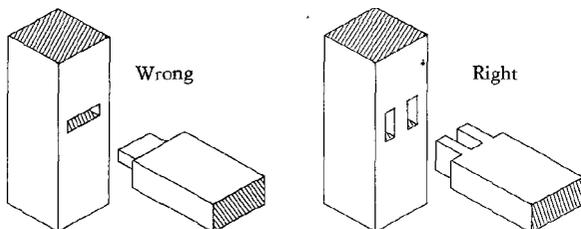
then the cheeks glue into end grain which is not a glue surface. The way to fasten narrow tenons is to use double (or triple) tenons, running the mortises in the direction of the long grain to provide good glue surface.
