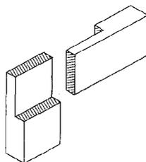
creased greatly because of the stop-action of the shoulders. Now double the surface area of the glue by making a slip joint
