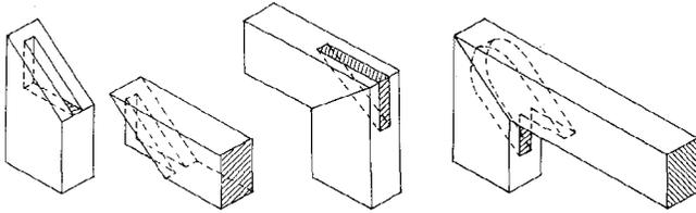
a spline is used purely for visual effect. The spline can also be hidden.
