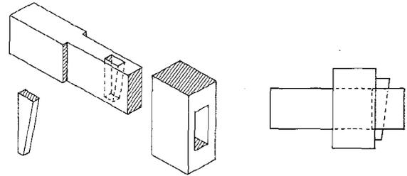
for the same effect. If the piece which receives the wedge is too thin, the two shoulders could be placed on the top and bottom instead of the sides.
