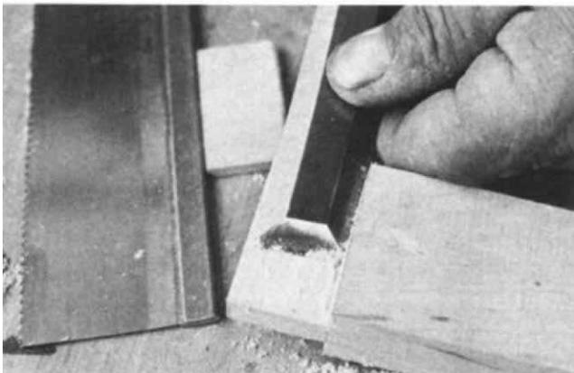
off the tenon corners slightly for easy insertion. Then sand the edge of the tenon so it will fit into the slightly shorter mortise.
