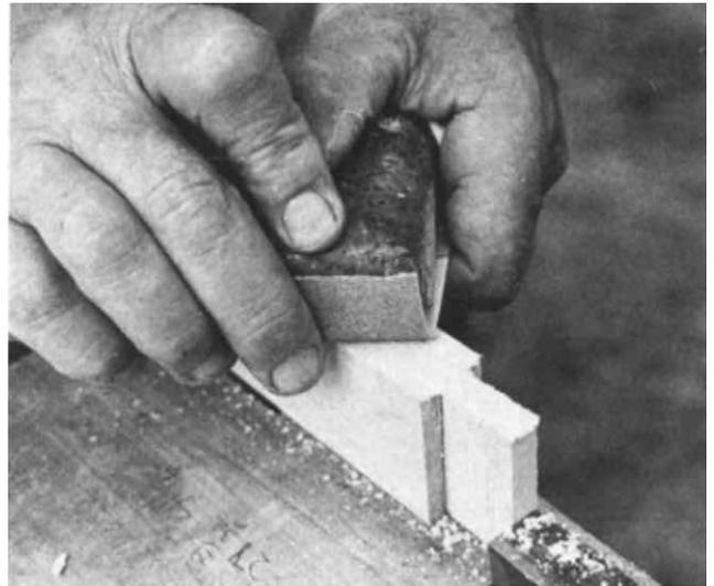
Now finish making your mortise. Take a small chisel and mallet to square off the corners, and a wide chisel (but no mallet) to flatten out the sides. Sand the outside edge of the
