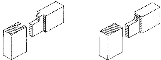
haunched mortise, or to a mitered haunched mortise where the tenon is completely hidden.
