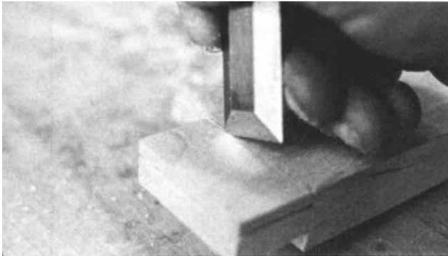
drawing the chisel along it. Then take a second cut at an angle to create half a "vee". You can then use this notch as a guide for your dovetail or frame saw. Finish sawing the shoulders and use a flat chisel to clean up the cheeks, and then round
