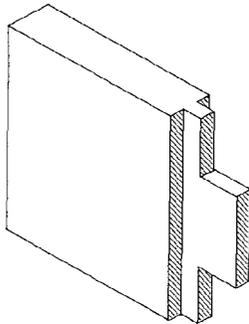
requires extra clamps for gluing the cheeks. But the haunches are necessary to keep the wood from twisting.
