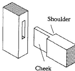
the tenon, which is the projecting part of the joint. One can imagine two crossed boards glued together. Despite the holding power of the glue, they can be twisted apart relatively easily.
