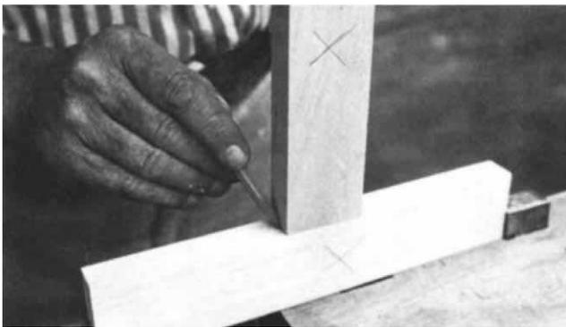
the tenon piece on the mortise piece, but I use a square to put lines just inside (less than 1/16-inch) those marks, because the mortise should be made slightly smaller to allow for subsequent sanding of the tenon.
