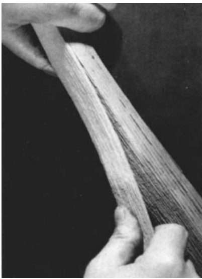
Basket-makers take advantage of weak earlywood (after pounding) of quarter-sawed ash to separate it into strips (left). Severely raised grain on pith side of flat-sawed hemlock (center) results from harder latewood being compressed into softer earlywood during planing, then springing back later. Honeycomb checks in red oak (right) can cause failure along large ray.
