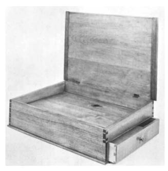
**Desk Parts** Large End  $3/8 \times 4-3/8 \times 12$ Small End  $3/8 \times 2 - 1/8 \times 12$ Back 3/8 x 4-3/8 x 18 Front  $3/8 \times 3-3/4 \times 18$ Bottom 1/4 x 12-1/2 x 18-1/2 Shelf  $1/4 \times 11-1/2 \times 17-1/2$ Top  $3/8 \times 12 - 3/8 \times 18 - 3/4$ **Drawer Parts** Front  $3/8 \times 2-1/8 \times 11$ Molding 1/8 x 1/2 Sides 1/4 x 2-1/8 x 17-1/2 Back  $1/4 \times 1-3/4 \times 10-5/8$ Bottom  $1/4 \times 10-5/8 \times 17-1/2$
