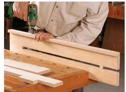
**Assemble the lip and face.** After the base of the fence is grooved, the lip and face are screwed in place.
