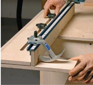
Each fence extends outward by 15 in. That's helpful when you want to set up the stop for extralong workpieces. A short shelf on each end supports those long boards (and cutoffs).
