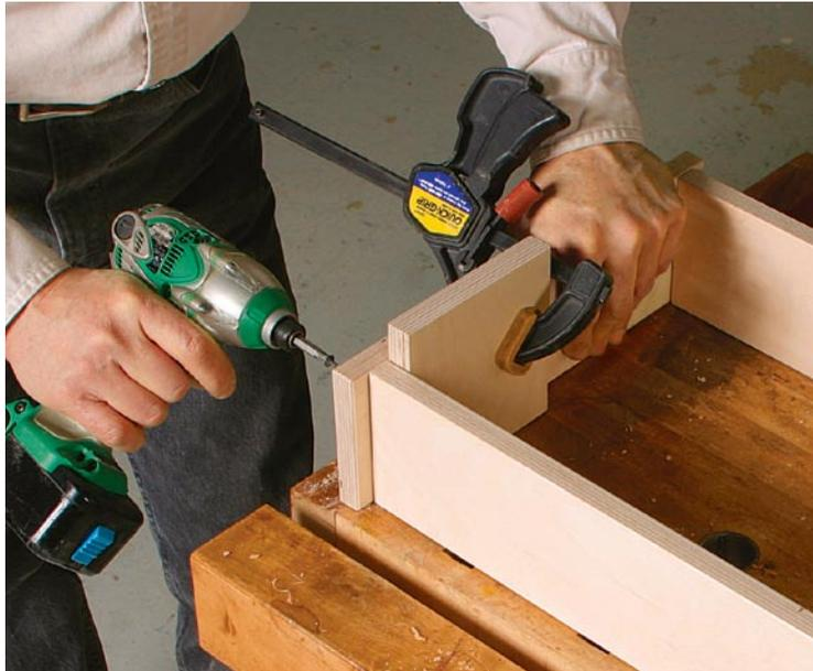
base. Use solid stock so you can plane down the blocks until the miter-saw table is flush with the stand tables. Using filler blocks here gives you some room for height adjustment if you happen to replace your saw.
