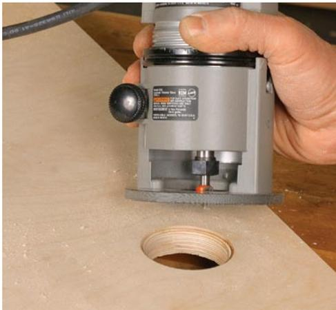
**Quick work.** White uses a trim router with a ¼-in.-radius roundover bit to soften the edges on all the parts, including the holes drilled in the front and back of the base.
