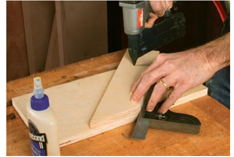
Pinned down. A few strategically placed brads keep the parts from shifting during glue-up.
