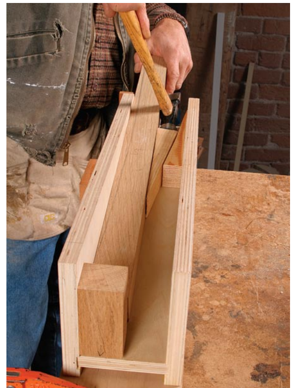
Low-tech hold-down. Opposing wedges can be an effective way to hold a workpiece in place in a jig like this router mortising box.
