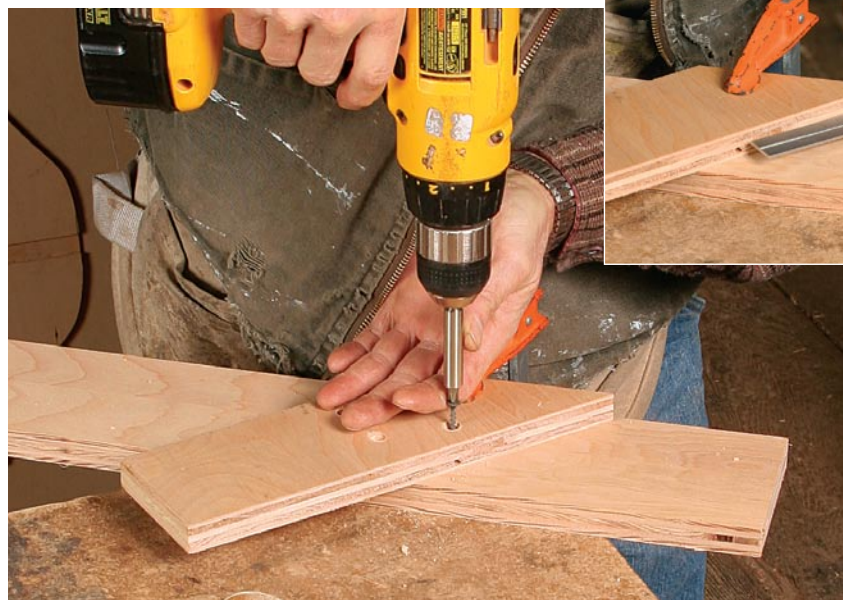
Clamp in place. Clamp components together to ensure that they are properly aligned (above). Keep components clamped as you drill holes and drive screws (left) to be sure the pieces don't shift.
