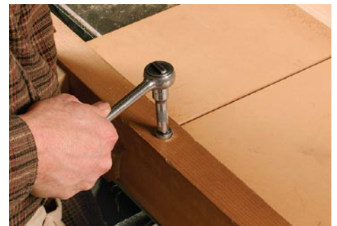
Wiggle room. Use bolts and slightly oversize holes when you need room for adjustment, such as on this crosscut-sled fence.
