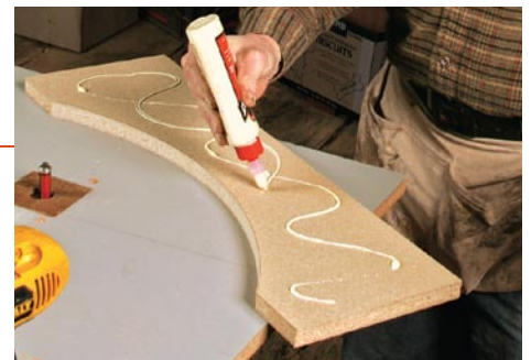
Glue for keeps. For jigs that will see repeated use, glue the components together.
