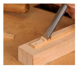
Long strips make it easy to manage small parts. Draw the profile on the stick, cut the shape on the bandsaw, and refine it with a chisel, keeping the extra length as long as possible.
