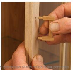
Install the pull as one unit. Glue the bail to the posts, and, before the glue sets, glue the whole pull assembly into the door stile.
