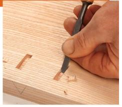
**Chisel the mortise into a ramp.** This gives the end of the friction catch somewhere to go as the door hits against it.
