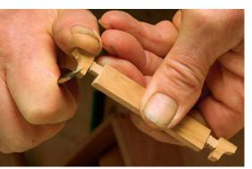
**Double-sided stick is easy to hold.** Use a small knife to detail the edges and corners, and use a chisel or tablesaw to cut the slight shoulders on the sides.
