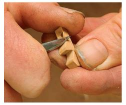
**Use a knife to chamfer all the sharp edges.**After using a handsaw to cut the catch free from the long stick, detail all the edges and corners as desired.
