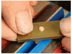
Perfect the size and shape of tenons. Having a 5/32-in.-dia. test hole in a scrap of hardwood or brass can be helpful during this process.
