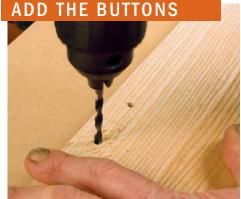
**Drill for the buttons.** The buttons are made from hardwood dowel stock. Round the tips slightly and glue them in.
