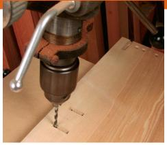
A place for the spring. On the drill press, create a small hole in the front of the mortise for a piece of spring (available at auto-supply stores).
