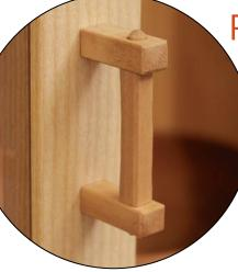
Two posts and a bail combine to make a subtle pull. Start by making the posts, and then create a bail to fit them. Pillow the ends of the bail tenons so they have a nice appearance and feel as they protrude through the holes in the posts.
