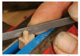
Cut the supports free and size the tenon. Carefully clamp the support into a small vise and round out the tenons using a sharp knife and small files.
