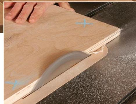
**Rotate and rip again.** Spin the piece around, putting the freshly cut edge against the fence and keeping the good side up in case there is slight tearout (left). Reset the rip fence and trim the piece to final width (right).
