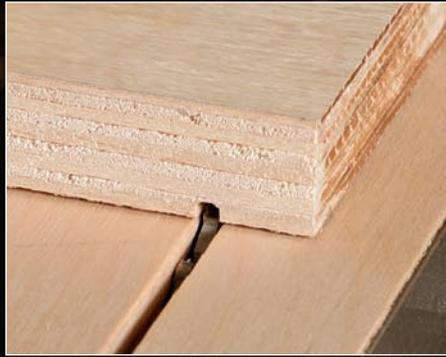
**Two techniques.** A sled ensures that you'll make safe, square crosscuts. To avoid tearout, either put tape over the cut line on the bottom of the piece (above left) or make a shallow scoring cut (above right) followed by a through cut.
