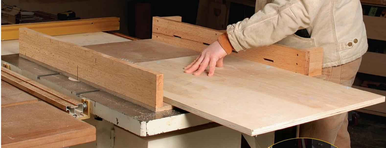
by ripping pieces  $\frac{1}{8}$  in. to  $\frac{1}{4}$  in. oversize, with a factory edge against the rip fence. Rotate the piece end for end, reset the rip fence to the exact size, and rip the piece again. This yields two clean, parallel edges. There won't be much tearout when ripping along the grain lines.
