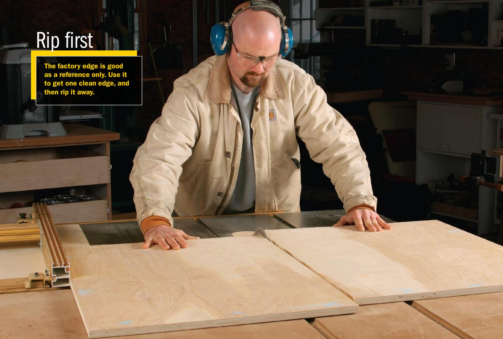
**Get one clean edge.** With a factory edge against the rip fence, cut the piece slightly oversize.
