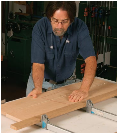
Press and rub. Place the glued edge against its mating edge and slide the two surfaces back and forth to distribute the glue evenly.
