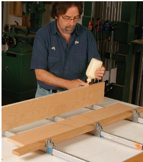
Don't spare the glue. Van Dyke applies a generous bead of glue on one edge, spreading it out with his finger.
