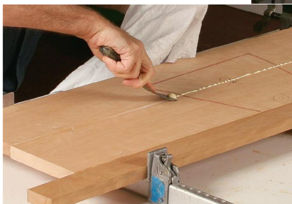
Easy cleanup. Before putting on the top clamps, scrape off most of the surplus glue with a putty knife.
