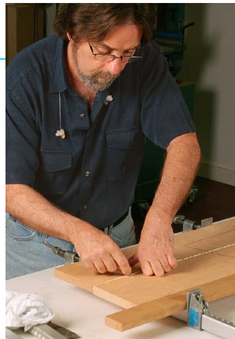
Align and clamp. Apply light force, aligning the surfaces with your fingers. Use a caul on the face that will be glued to the other half.
