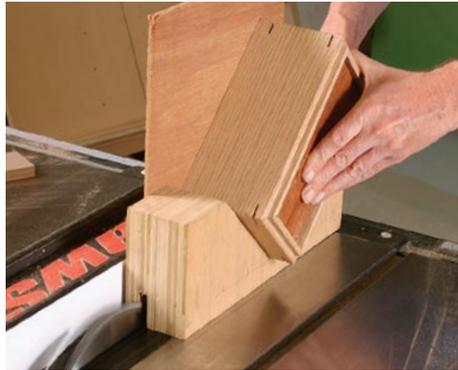
**Good for joinery.** Made for ripping and crosscutting, a blade with a combination grind (ATB and FTG teeth) will leave a kerf with a nearly flat bottom. This is useful for joinery. In this example, it leaves no visible gap between the spline and the box.
