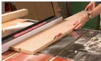
**Ready for glue.** The Glue-Line Rip Blade from Freud (item No. LM74R010) is designed to leave supersmooth edges that won't need jointing—but only on boards up to 1 in. thick. The 30 teeth alternate between FTG and triple-chip grind (TCG).
