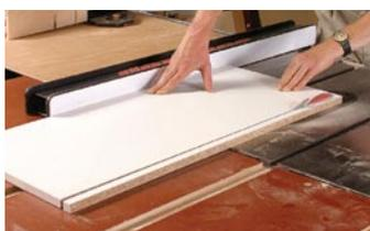
**Clean cuts for the long haul.** If you cut large amounts of double-sided laminate or melamine, the 80-tooth TCG blade makes cuts that are almost as clean as a high-ATB blade, but is more durable.
