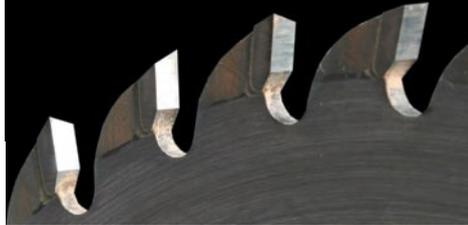
**Cleaner cuts.** Most all-purpose blades have only ATB teeth. A combination-grind blade has one FTG tooth between four ATB teeth, which reduces vibration.
