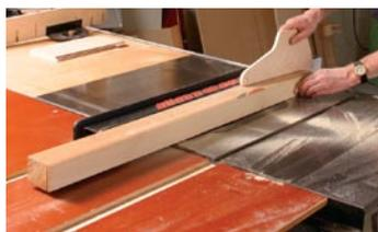
**Big teeth, far apart.** A typical 10-in. rip blade has 24 teeth, each with a flat-top grind (FTG) and a hook angle of 20° to 25°, which helps pull the stock into the blade. The deep gullets help clear the large volume of chips created by ripping. A rip blade will cut thick stock far quicker than a combination blade and with less user effort.
