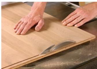
**No tearout.** Some sheet goods are notoriously difficult to crosscut cleanly. A high-ATB blade cleanly shears the most brittle of veneers. However, the sharp tips on the teeth of a high-ATB blade are more easily damaged than those on rip or combination blades.
