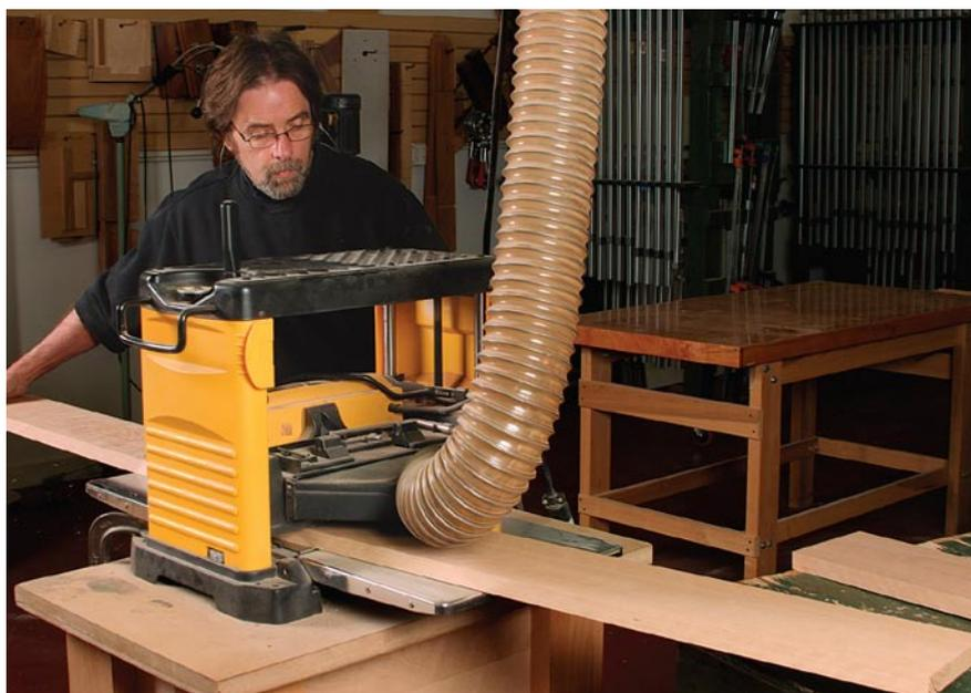
**Plane the other face parallel.** Run the boards through the planer until the face opposite the jointed one is just smooth. Don't aim for final thickness yet.
