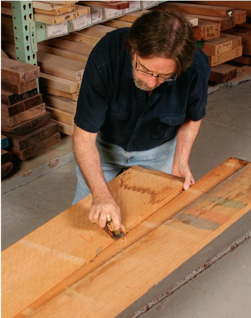
**Sneak preview.** At the lumberyard, if the boards are roughsawn, ask permission to block-plane a small section to get a better view of the wood's color and grain.
