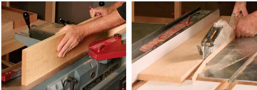
**Joint one edge, then rip to width.** Run one edge over the jointer until it is flat and at 90° to the face that is against the fence (left). With the jointed edge against the fence of the tablesaw (right), rip each board slightly over final width.
