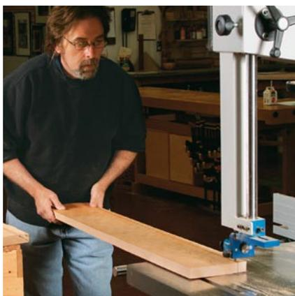
**Bandsawing is safer.** Ripping the unjointed boards on the tablesaw might cause kickback. So cut them  $\frac{3}{4}$  in. over final width on the bandsaw.
