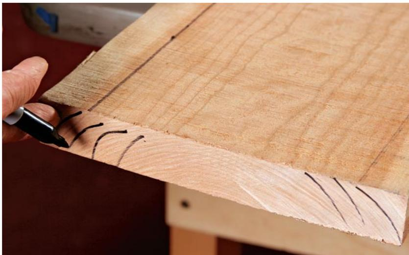
**Riftsawn edges add stability.** Try to find boards where the growth rings run at about 45° to the face where the finished edges will be. This ensures that the sections of the top will stay flat.
