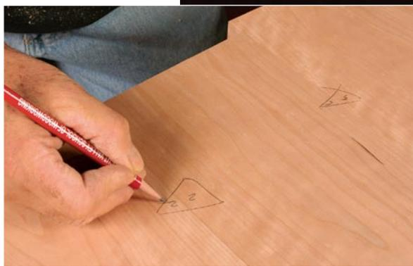
**Record good matches and make the final choice.** When you find two boards that go well together, draw a small triangle across the joint and number both sides (above). This will make it easier to come back to this pairing after you've tried other combinations. After you have found the best sequence of boards, draw a large triangle across the whole top (right).
