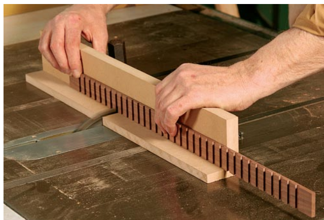
Cut accurate dados. The twin-gauge setup works well for making cuts across the middle of a long workpiece. Used miter gauges are inexpensive and easy to find at flea markets or online.
