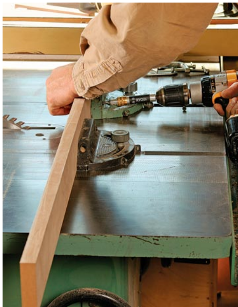
Two gauges run side by side. One sits in each slot; together they support a long fence.
