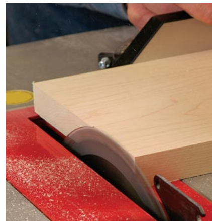
No deflection on trim cuts. Even when the thin-kerf blades weren't buried in the cut, they made smooth and square cuts. That's impressive, because an unsupported blade can deflect away from the board, causing a rough and out-of-square cut.
