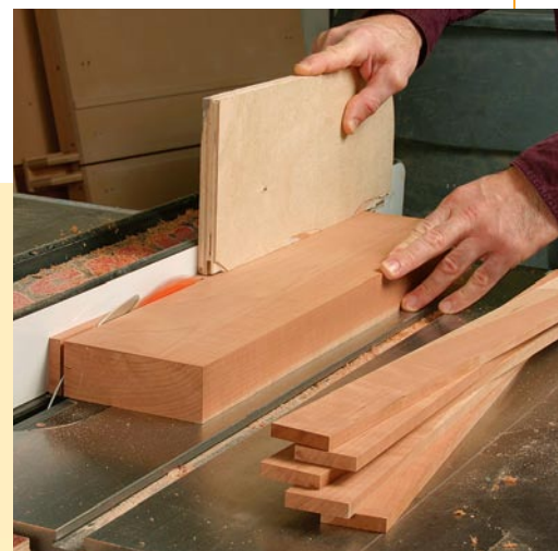
No deflection on trim cuts. Even when the thin-kerf blades weren't buried in the cut, they made smooth and square cuts. That's impressive, because an unsupported blade can deflect away from the board, causing a rough and out-of-square cut.
