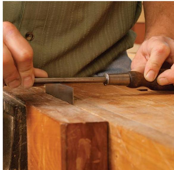
Use the burnisher at an angle of 1° to 15° to flatten this ridge and create a hook-shaped cutting burr. A steeper angle yields a more aggressive cut.
