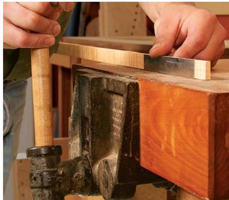
**2 Turn the burr.** Use a piece of scrap as a reference to set the scraper's edge at a consistent height. Then ride the burnisher's handle along the bench to maintain a consistent angle, and make several firm pushing strokes away from you.
