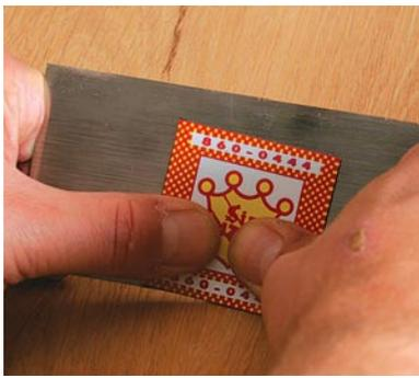
**Two thumbs down.** Grasp the scraper with your fingers wrapped around each side and your thumbs together on the back, near the bottom edge. Push forward with your thumbs, applying enough pressure to create a slight bow. The more pronounced the bow, the more aggressive the cut.
