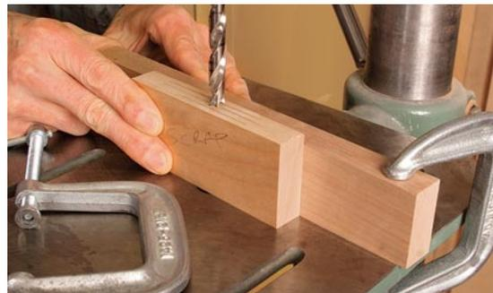
**Drill press does the grunt work.** Use a bit that matches the mortise width. Clamp a fence to the table to ensure that the bit drills into the center of the piece.
