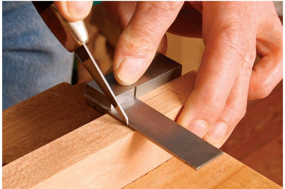
**Scribe the ends.** To complete the layout, use a knife to scribe a cut line at each end of the mortise.
