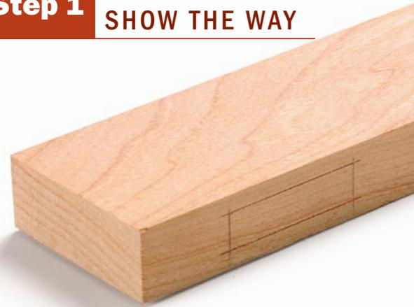
**Scribe the sides.** After marking the location with a pencil, use a marking gauge to scribe each side of the mortise, stopping at the pencil lines.
