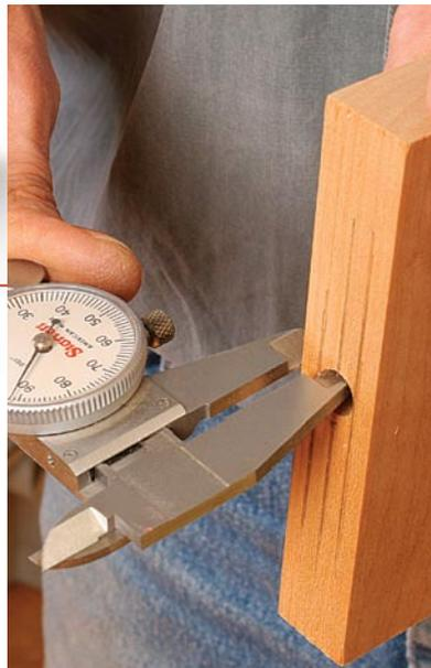
**Dial it in.** After drilling a single hole in the test piece, use a dial caliper to make sure the hole is centered.
