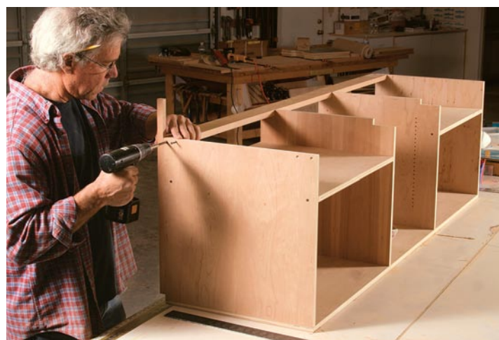
Solid-wood stretchers connect the piece at the top. These also create a place to attach the back and top of the cabinet. The front stretcher protrudes \frac{3}{4} in. from the case, to meet the other edging, so Casey uses a piece of \frac{3}{4} -in. scrap to set the reveal.
