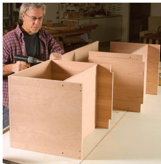
The fixed shelves are first. Construction begins with two H-shaped subassemblies (above). These assemblies are then connected by a plywood bottom (left). The space between them creates the central shelving area.
