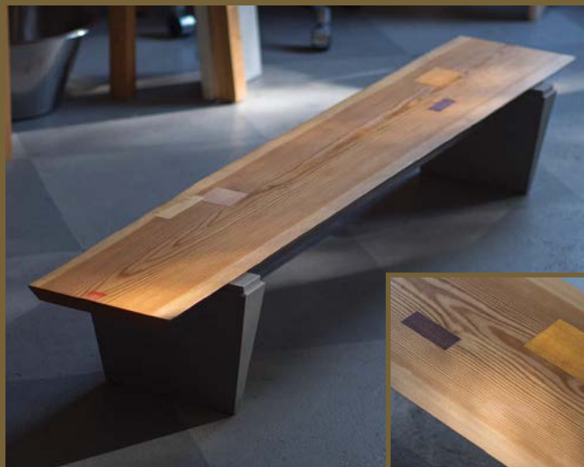
Playful patchwork. The seat of Aramburu's bench features inlaid and stained patches of pine and spruce, randomly placed in a plank of Swedish pine. The legs and stretcher, also solid pine, are coated with milk paint.
