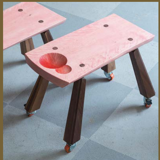
Traveling table and stools. The side table in ash, with milk-painted stretcher and tusk tenons, was made to be flat-packed. Tapered sliding dovetails join its thin legs and top. The jaunty stools with staked legs are a mobile take on a traditional milking stool.
