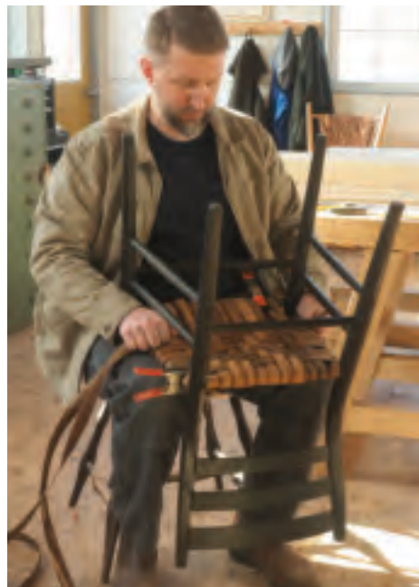
Weave the seat. Once you've harvested the hickory bark, weaving the seat is the easy part.
