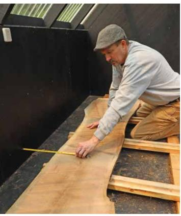
**Keep the airways open.** When laying the first board in a load of lumber, Plourde makes sure to space it 12 in. from the knee wall so the circular airflow around the stack, critical to even drying, is unimpeded.
