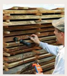
**Meter man.** Plourde uses a pin-style meter to document the lumber's moisture content before and during the drying cycle. This load went in at 17% MC and emerged five weeks later at 8%.
