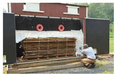
**Totally baffled.** Once the lumber is stacked and the fans are hung, Plourde staples up baffling material to close off the openings around the stack. This ensures that the air heated by the sun and driven by the fans will be drawn through the stack of lumber, drying it quickly and evenly.
