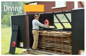
**Critical fans.** Two inexpensive car-radiator fans, each powered by a solar panel, circulate the air in the kiln. Mounted on plywood that hangs by French cleats, the fans are easily removeable for loading and unloading. Quick-connect couplings to the solar panels speed the process.
