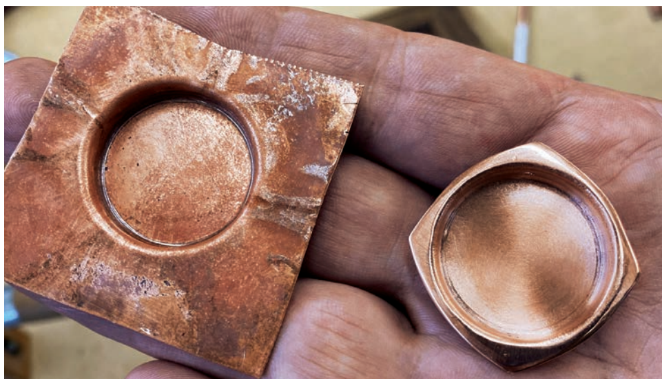
Sweet transition. After tapping out the wrinkles, Cullum trims the skirt with snips, smooths the edges with a file and abrasives, then polishes all surfaces. He also drills two small holes for nails in the side wall of the recess.
