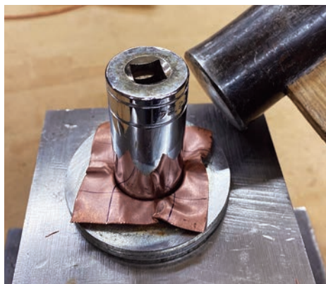
Homemade punch press. With a sacrificial socket wrench socket and a couple of big washers, Cullum devised a machine to emboss copper sheet for finger pulls. After pounding, he carefully taps out the wrinkles in the skirt around the recess.
