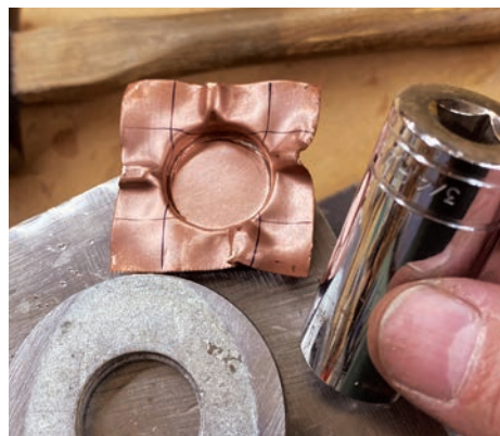
Homemade punch press. With a sacrificial socket wrench socket and a couple of big washers, Cullum devised a machine to emboss copper sheet for finger pulls. After pounding, he carefully taps out the wrinkles in the skirt around the recess.
