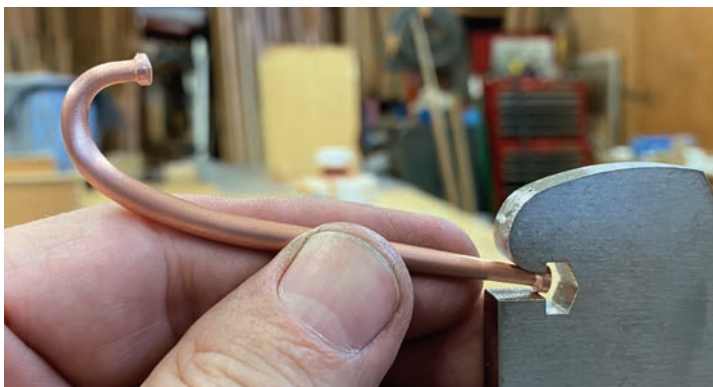
The bail gets finished and fixed. After completing the bend, Cullum polishes the bail, then adds at each end a cotter pin with a customized copper washer. He gives the washers their domed shape with a dapping block.
