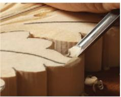
**Lower the leaf.** Using a #7–6mm, start with a vertical stop cut along the layout line (left). Follow up by angling the gouge 45° and carving toward the stop cut (right) so the leaf tip looks like it's curling under.
