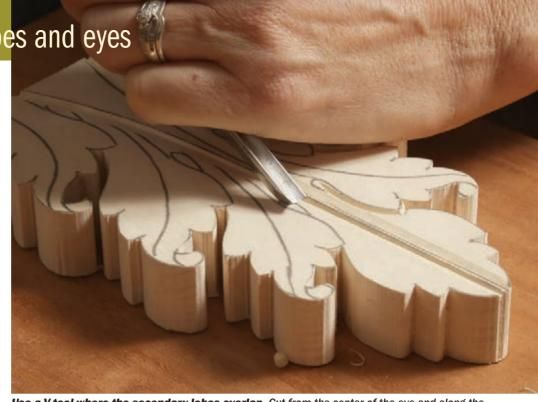
**Use a V-tool where the secondary lobes overlap.** Cut from the center of the eye and along the edge of the overlapping lobe. Make sure you leave the line visible, and that you cut on the side of the lower lobe.
