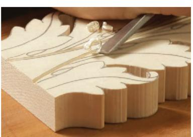
Lower the leaf near the middle vein. Use a #3-14mm gouge, holding it bevel down while gently rounding it away from the vein until about ½ in. into the leaf. A bench chisel held bevel-down will also work.
