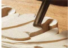
**Notch the serrations using a thumbnail cut.** Carve these serrations with two cuts using a #7–6mm. Start with a vertical chop that continues the serration into the leaf, then angle the gouge to remove a small triangular chip. This should give the appearance that the lobes slightly overlap.
