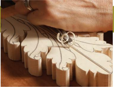
Use a V-tool along both sides of the middle vein. These cuts should start ½ in. deep but get shallower as they reach the tip of the leaf. Make several passes to reach the full depth and ensure clean, sharp edges.
