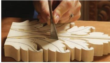
**Define the secondary lobes' upper edge.** Make a vertical cut directly on the line. Use a #5–14mm for the longer sections and #3–6mm for the smaller sections. These cuts should connect with the eye's walls.
