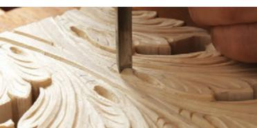
Use thumbnail cuts below each eye. Use a #7-6mm to cut a pair of wrinkles under each eye using the two-step thumbnail cut. These should get slightly smaller as they go down the pipe.
