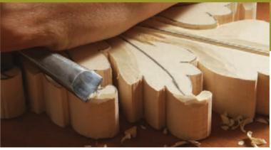
Round over the outer edges of the curling leaf. Use a #3–14mm and mind the grain direction. Take multiple smaller slices to maintain control.
