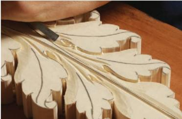
Carve along the pipe. With a #11-3mm gouge, make two sweeping cuts down the leaf to define the pipe. These cuts should start on either side of the eye, and converge as they reach the middle vein (top). In this design, these cuts also extend and curve around the eye to begin shaping the leaf detail. Round over any sharp corners with a #3-6mm gouge (bottom).
