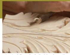
**Hollow the lobes.** The #8–10mm gouge's sweep creates good dimension in the lobes. Lower the middle of the lobes in multiple passes if necessary to maintain a clean, crisp surface. The lobes' sharp, raised edges should follow the curve of the leaf and gently flow toward the base of the leaf along with all other lines.
