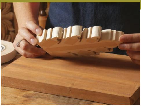
**Secure the blank to a backer board with double-sided tape or a paper joint.** This lets you clamp the backer board rather than the carving, giving you full, unobstructed access to the leaf.
