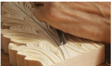
Create the veins in each lobe. Use a #11-2mm and make sure the veins curve gently down the leaf and fade off without overlapping.
