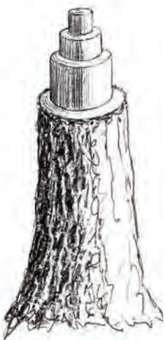
Growth rings, which are added in annual sleeves, nest in layers, as can be seen on the surface of a flatsawn board.
