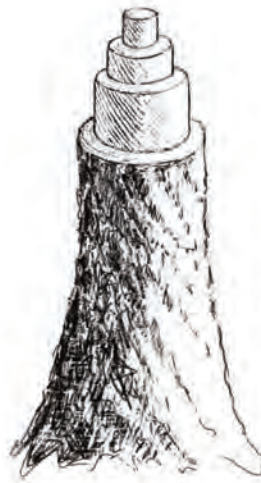
A flatsawn plank cut from a twisted tree will have a similar grain pattern on its surface. The twist is only revealed when the wood is split—or the woodworker attempts to plane the surface!
