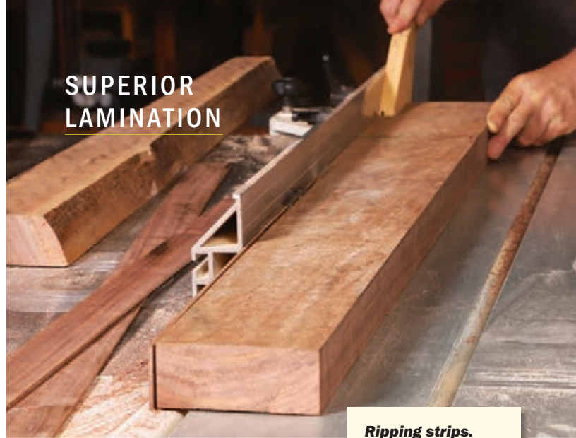
Ripping strips. Even thin parts will have fibers running their full length. With their excellent strength and flexibility, thin strips that follow the fibers are well suited for bent lamination.
