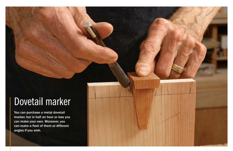
Quick to make. Starting with an over-length piece of stock, establish the shoulders on the table saw. Then cut the cheeks at the bandsaw. While the stock is still long, pencil in your angle lines, and then cut them freehand on the bandsaw. A handsaw would handle these tasks as well. Finally, crosscut the marker and refine the angles with a hand plane or sanding block.
