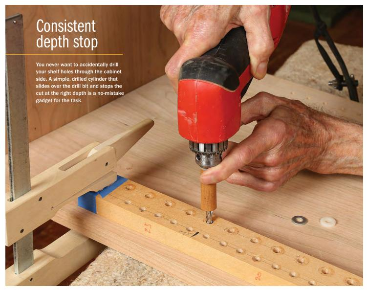
**Drill and trim to** length. Clamp your dowel tightly in a hand screw, and drill a hole the same size or slightly larger than the diameter of the intended drill bit. The hole you drill doesn't have to go all the way through the dowel. Then cut the dowel to length based on the desired depth of hole. You can fine-tune the depth of the holes you'll be drilling by trimming the stop or adding washers.
