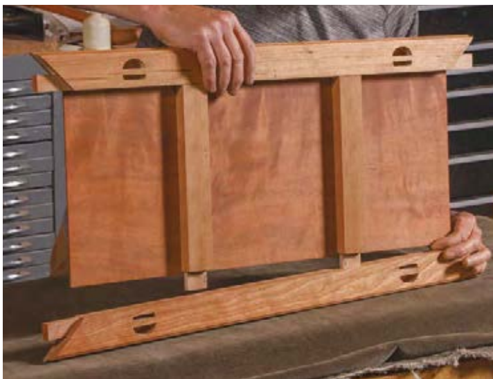
Back to the top. Once the cross braces are snug in their sliding dovetail sockets, Cameron fits their tenons into the long members of the top frame.
