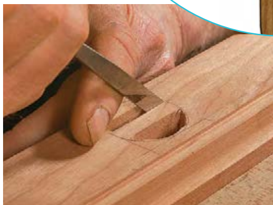
Half-moon mortise. Cameron uses an in-cannel gouge to shape the rounded wall of the outer mortise. He'll use a smaller gouge to round the ends of the inner mortise.
