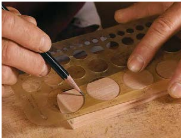
Coping with the tenons. The frame members get tenons with coped shoulders that wrap around the leg. A circle template helps lay out the coping.
