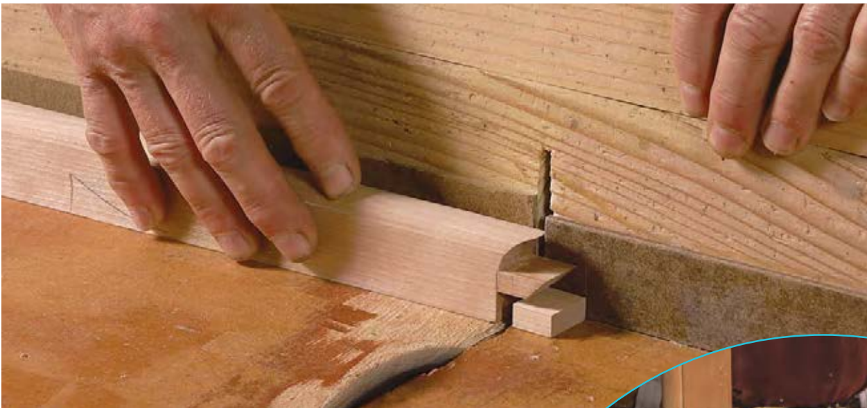
Ensuring one flat shoulder. The tenons on the short frame members are cut next. They have a coped outer shoulder to wrap the leg, but their inside shoulder is not coped, and Cameron cuts it at the tablesaw. A spacer clamped to the sled skews the workpiece, making the cut 1.5° off square.
