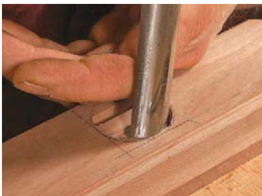
Half-moon mortise. Cameron uses an in-cannel gouge to shape the rounded wall of the outer mortise. He'll use a smaller gouge to round the ends of the inner mortise.
