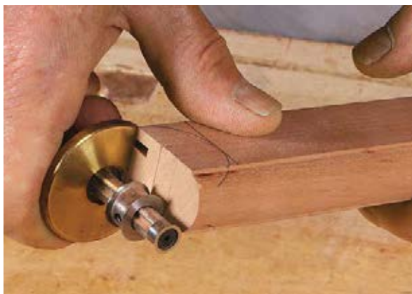
Tenons get scored. Using a marking gauge with a double cutting wheel, Cameron marks the tenons using the inside edge of the workpiece as his reference surface. A regular gauge will also do the job.
