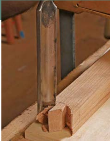
Curved cleanup. The in-cannel gouge is key as Cameron pares the coped shoulders and then fits them to the leg.
