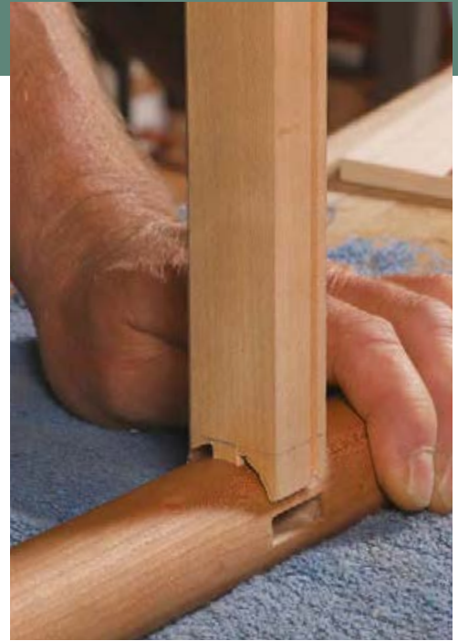
Ensuring one flat shoulder. The tenons on the short frame members are cut next. They have a coped outer shoulder to wrap the leg, but their inside shoulder is not coped, and Cameron cuts it at the tablesaw. A spacer clamped to the sled skews the workpiece, making the cut 1.5° off square.
