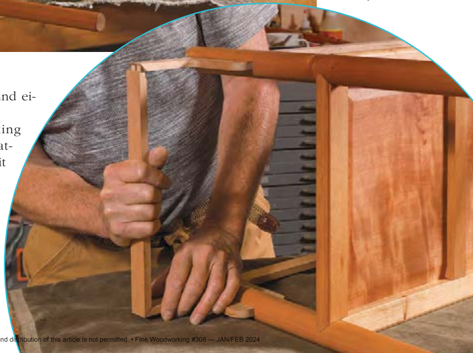
Dovetails get a little leeway. There should be just enough flex in the assembled structure to let you widen the gap between the long aprons and sneak the short apron into place.
