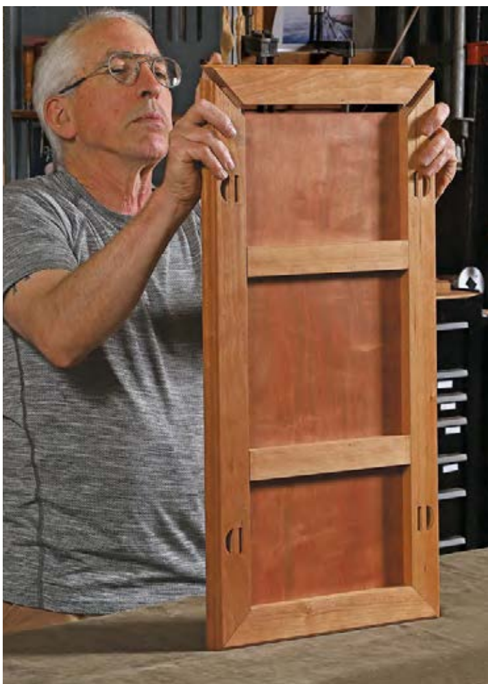
And at the end. The short members of the top frame slide on last, and the through-tenon joinery locks the cross-brace tenons tight.
