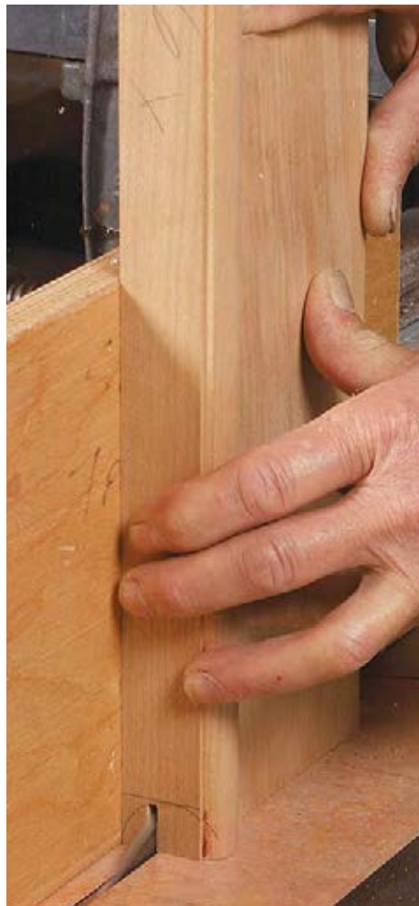
Complex tenon starts with a simple cut. To anchor the cutting with a solid reference surface, Cameron cuts the inside cheek at the tablesaw, using a high fence and a square following block. Then it's on to handwork.
