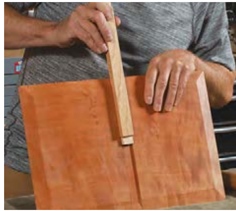
The shelf itself. With its wide underbevel and its sliding dovetail slot, the shelf receives a single cross brace. Once the panel is in place and the cross brace is fitted, Cameron adds the short frame members.
