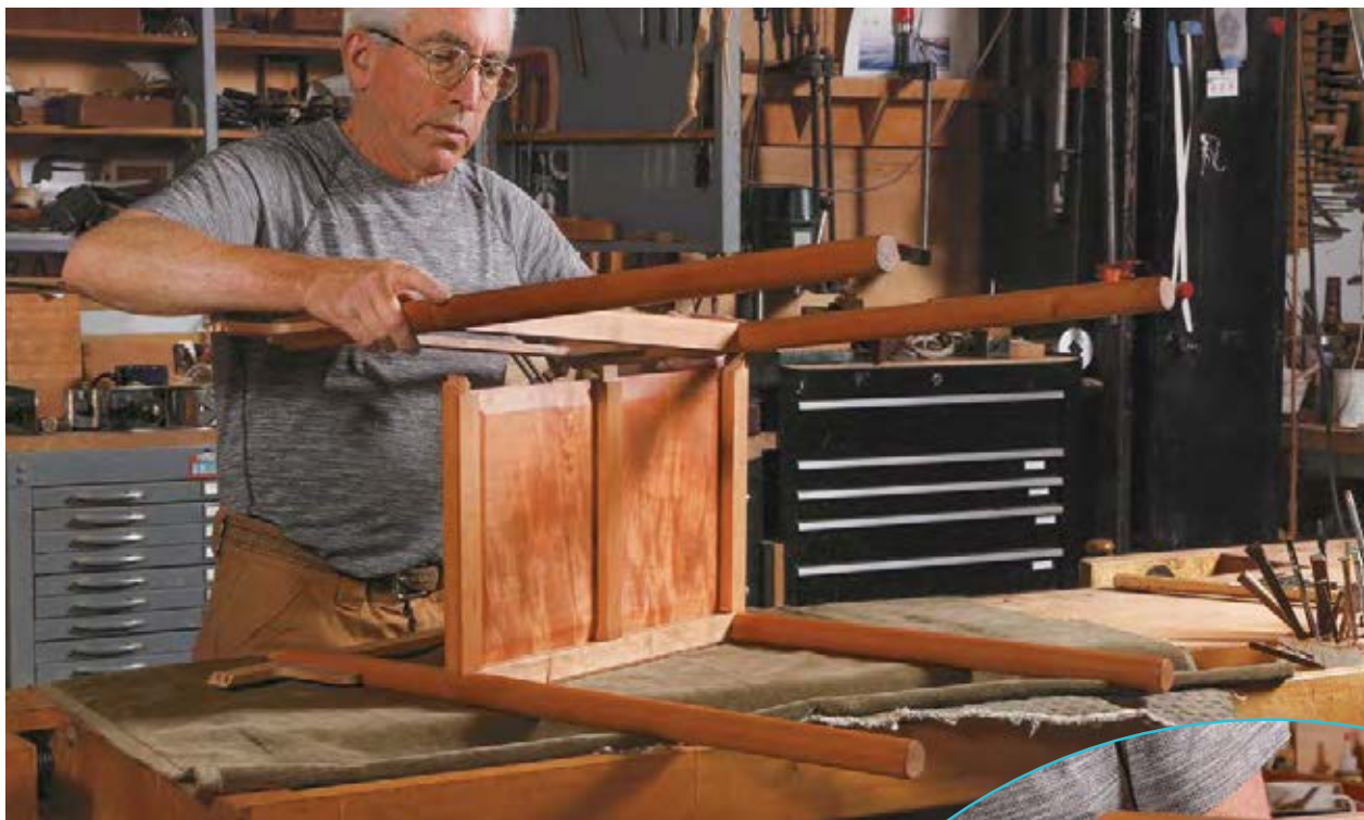
Two more legs. The second pair of legs, with apron and long shelf frame in place, completes the shelf assembly.
