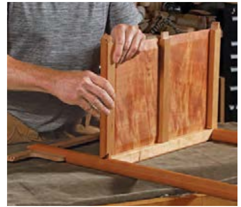
The shelf itself. With its wide underbevel and its sliding dovetail slot, the shelf receives a single cross brace. Once the panel is in place and the cross brace is fitted, Cameron adds the short frame members.
