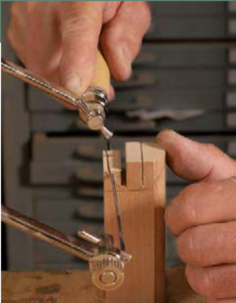
Long members first. The front and back frame members are coped to embrace the leg with both shoulders. Cameron makes the curving cuts with a coping saw.
