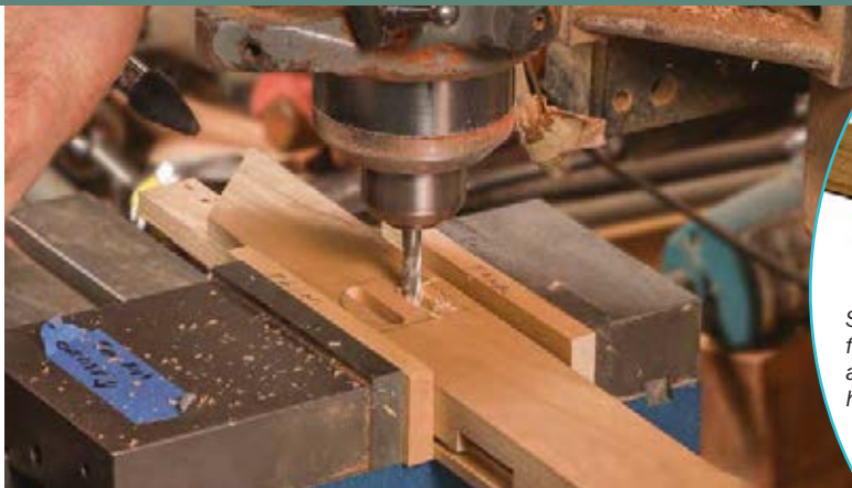
Milling a double mortise. The oddly shaped twin mortises in the top frame to receive the leg tenons begin with a pair of ordinary, machine-cut, side-by-side mortises.
