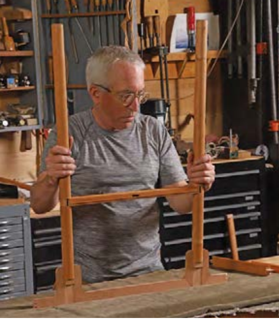
Legs to apron. After fitting the long shelf frame member between two legs, Cameron slides the legs onto the spandrels.
