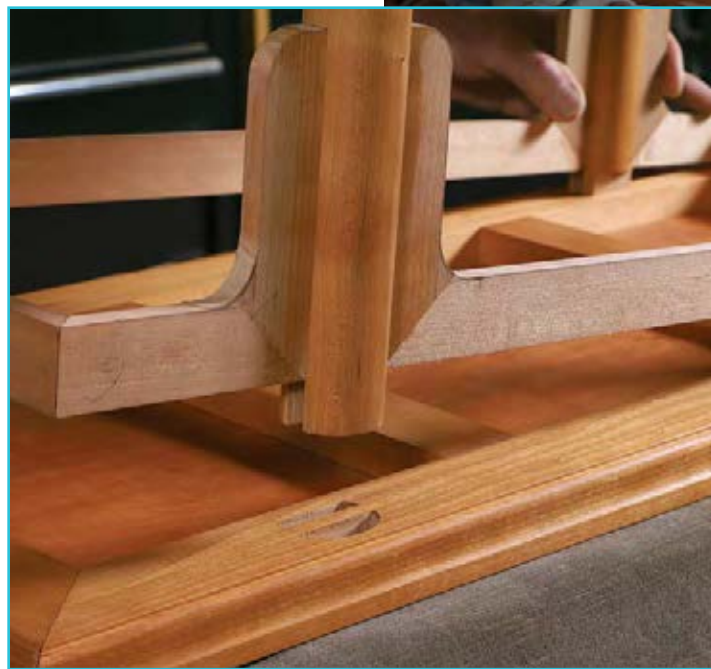
Tipped and tapped. With the top upside down on a clean, cushioned surface, Cameron tilts the base a bit to nudge one set of legs into their mortises, then lowers the other set. Because the legs splay and the mortises are slightly angled to match, the top won't lift off once the base has been tapped all the way home.
