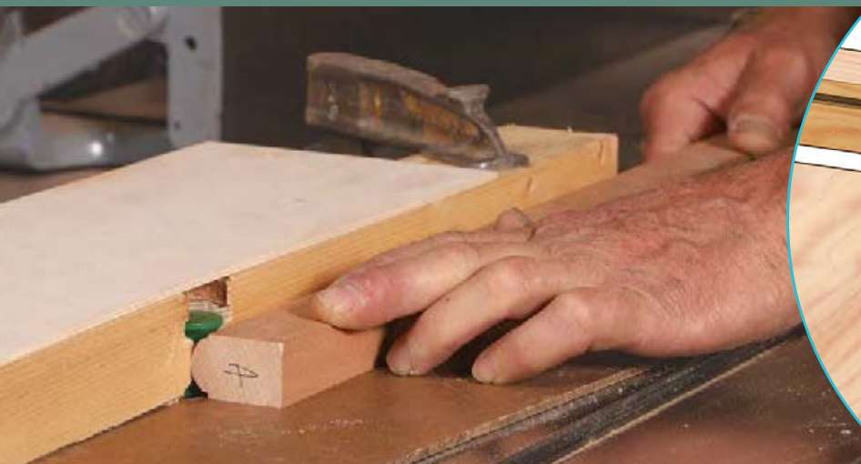
Molding and grooving. With the shelf's frame stock milled to size, Cameron cuts the molding profile on the router table with a half-radius bullnose bit, then a thumbnail beading bit. Next, at the tablesaw, he'll cut a 1/8-in. groove to accept the panel's tongue.
