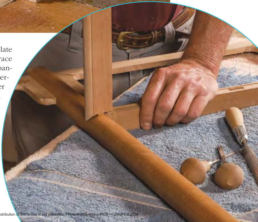
Ensuring one flat shoulder. The tenons on the short frame members are cut next. They have a coped outer shoulder to wrap the leg, but their inside shoulder is not coped, and Cameron cuts it at the tablesaw. A spacer clamped to the sled skews the workpiece, making the cut 1.5° off square.
