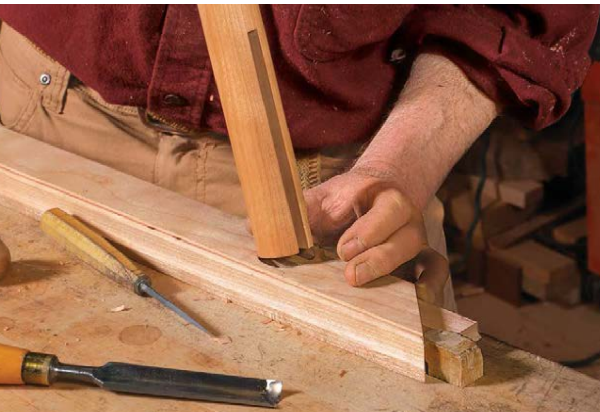
Half-moon mortise. Cameron uses an in-cannel gouge to shape the rounded wall of the outer mortise. He'll use a smaller gouge to round the ends of the inner mortise.
