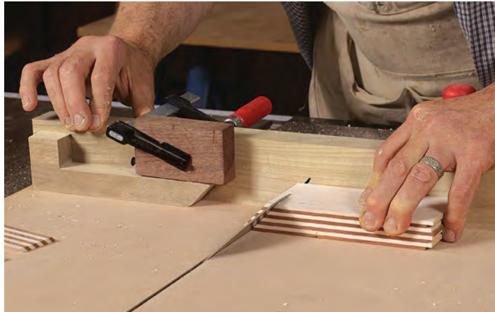
Angled crosscuts. A mitered L-stop allows the bricks to be cut at 45°. This opens up the possibilities of different patterns.
