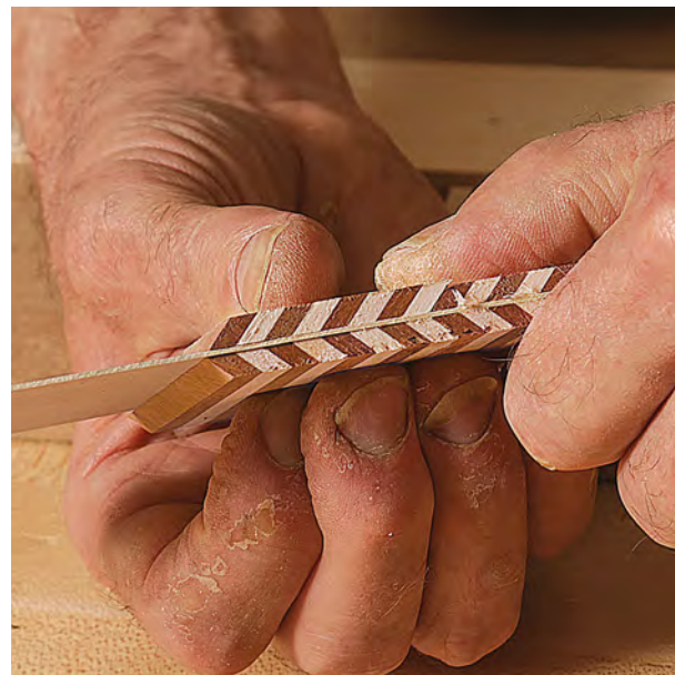
Laying up bricks. Side by side, the 45° pattern makes a beautiful herringbone pattern (far left). Placing veneer in between the bricks makes up a traditional arrowhead pattern (left).
