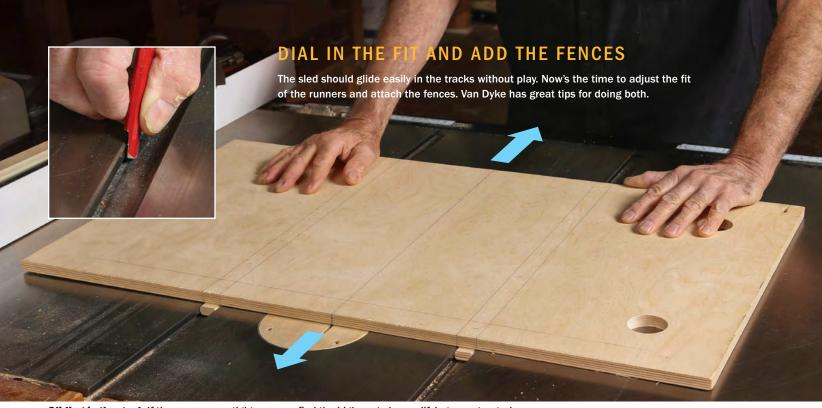
**Gliding is the goal.** If the runners are tight, you can find the high spots by modifying a contractor's pencil and rubbing graphite against the slot. Push the sled into the tracks and move it back and forth.
