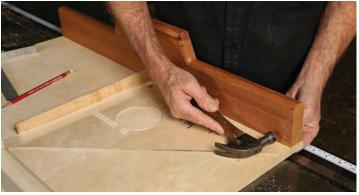
Add a spacer, and square up the fence. Wedge a spacer into the kerf; it should be a snug fit. Place an architect's triangle against the spacer and tap the fence until it is perfectly square to the spacer. Verify that your triangle is actually square.
