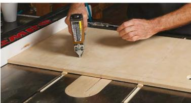
end of the fence layout and centered on the fence thickness. The depth should be just enough that the head of the screw does not protrude. Using the dimple left by the Forstner bit as a guide, drill a 3/16-in. hole centered in each counterbore. Using the same drill bit and a small chisel or a round rasp, elongate one of the holes—1/4 in. to 3/8 in. long is more than enough.
