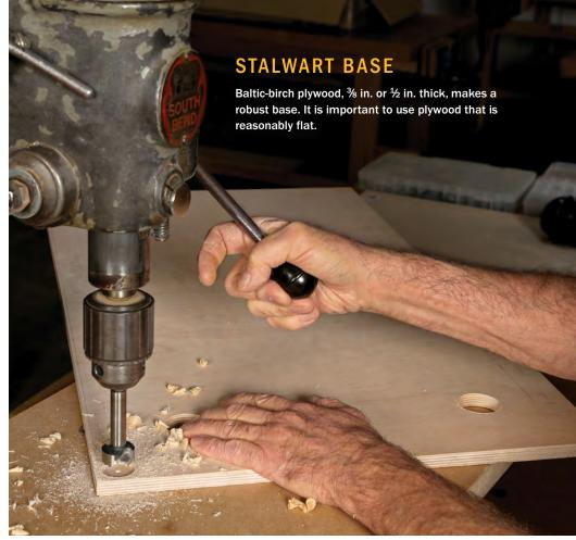
**Hanger holes first and foremost.** The first thing Van Dyke does to the base is to drill hanger holes. If you take care of the sled, hanging it on the wall when not in use rather than leaning it against a wall or machine or on the floor, it will last decades and stay in square.
