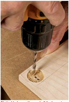
Slotted hole on other end of the base. In a second recess at the other end of the base, cut a slot by drilling three through-holes and chiseling out the waste between them. This will allow you to adjust the fence for square before permanently securing it to the base.
