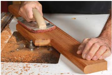
**Comfort first.** The fence's top piece keeps your hands away from the blade, supports work held vertically, and, once you've cut through the fence, it holds the two halves together. Round over the top edges to remove sharp edges and make the fence more comfortable to use.
