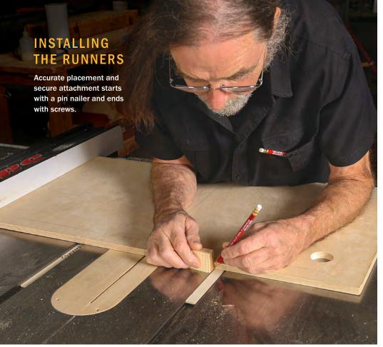
**Use the table-saw fence as a stop.** Set the fence to half the width of the base. Place the runners in the miter slots with spacers underneath to bump them up slightly. With the base pushed against the fence, use a square or a squared block to mark the location of the runners on the base. Carry those lines across the top of the base to guide the pin nailer in the next steps.
