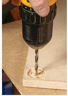
**Pivot screw on one end of base.** In a shallow recess made with a Forstner bit in the underside of the base, drill a clearance hole right through. This will accept a screw going into the bottom edge of the fence, allowing the fence to pivot on the base.
