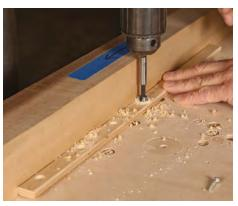
**Prep the runners for screws.** At the drill press, add a counterbore with a Forstner bit, and finish with a  $\frac{1}{6}$ -in. bit as a pilot hole as well as a clearance hole.
