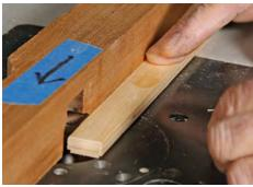
Mill the runners. After ripping strips of plywood to near final width, run them on edge through the planer to get them to exact size. Cut a small rabbet along the edges of the face that will meet the bottom of the sled, and gently round over the edges of the other face.
