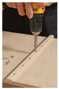
**Permanently attach the runners.** When the glue has dried, take the assembly out, turn it upside down, and screw the runners in place with round-head screws.
