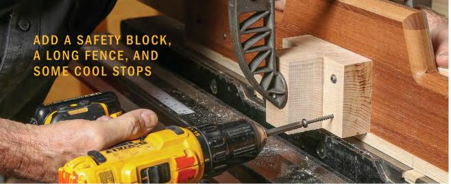
Attach a wooden exit guard. Don't neglect this simple safety device. When you use the sled, the blade will come right through the front fence. Your hand should never be near there, but just in case it is, this block will protect you from the blade.
