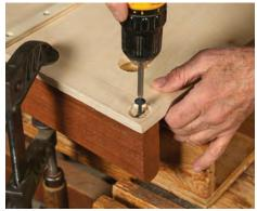
Temporarily screw the front fence in place. Clamp the fence to the base. From the underside, first drive the pivot screw, then drive a screw into the center of the slotted hole on the other end.
