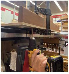
temporarily. Once you tap the fence square to the spacer, add a clamp, tighten the screw in the slotted hole, and drive a temporary screw an inch or two away to stabilize things.
