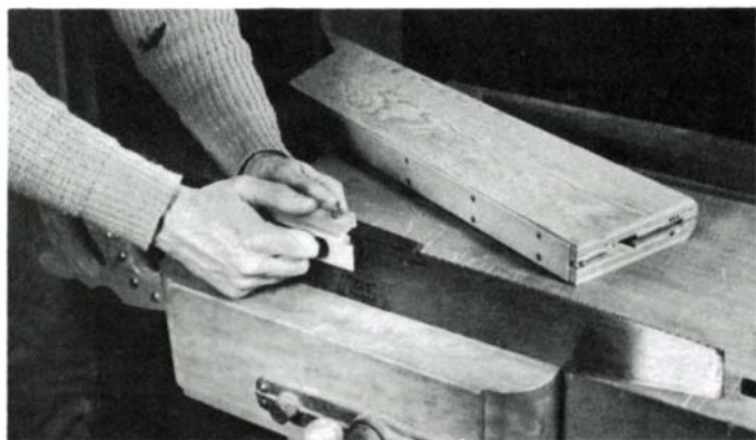
To joint the teeth, place the saw in the bench vise and a smooth mill file in the jointing guide. Hold the guide flat against the side of the blade and run the file gently over the top of the teeth. The saw vise pictured on the bench is used in subsequent steps.
