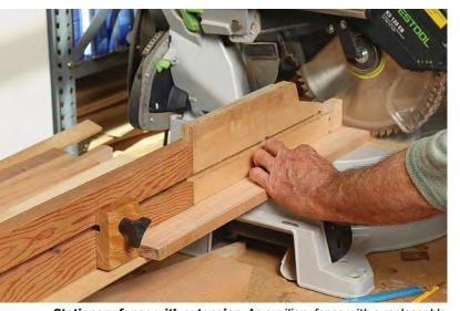
**Stationary fence with extension.** An auxiliary fence with a replaceable zero-clearance throat piece and a groove for an adjustable stop are the foundation for straight, square, repeatable cuts, without tearout. The removable extension fence locks onto either end of the stationary fence via dowels. It also has a ledge on the bottom to support the workpiece at the same height as the saw's table.
