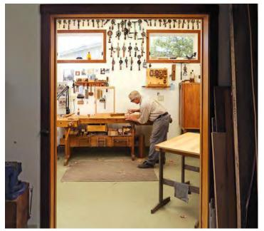
**Big enough.** Just over 150 sq. ft. with high ceilings and lots of windows, the bench room has enough space for a large bench, storage cabinets, lots of light, and open floor space for gluing up larger pieces and working on pieces in progress. The floors are gentle on the body, poured concrete with multiple layers of plywood on top and vinyl flooring tops it off.
