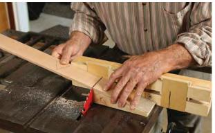
Versatile auxiliary fence. The shopmade add-on to the saw's miter gauge prevents tearout by backing up the cut with a replaceable insert. It also has an easily adjustable stop. A simple ramp held against the fence aids in crosscutting angles.
