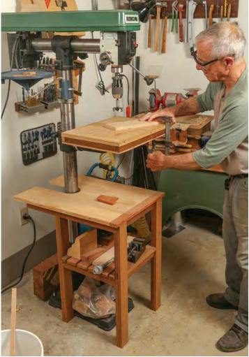
**Surround the factory table.** Welter built an auxiliary table that wraps around the drill-press table. This means he always has a flat surface to clamp to underneath. When the insert under the drill bits gets chewed up, he can slide it out and put in a new one rather than replacing the entire table (top photo). Welter also built a two-tier accessory table (above) that straddles the drill press's column; it is easily moved if greater depth is needed.
