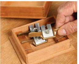
boxes. Welter makes custom boxes for hand tools that are special or seldom used. He tailors the size of the box and the cradles inside to the specific tool, and stores the boxes on a shelf.
