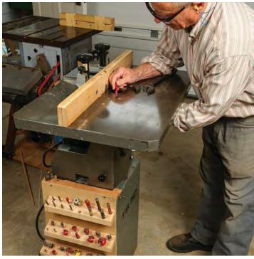
Keep your bits close. A bit rack on the router table keeps you from having to walk across the shop for bits. Drill the holes completely through, then drive nails into the board so one crosses each hole near its bottom. The nail supports the bit but lets dust and shavings fall through instead of collecting at the bottom of the hole.
