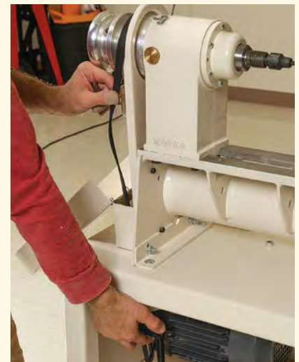
Easy change. The motor, which is located beneath the headstock, within the stand, has two speeds that are easily changed.
