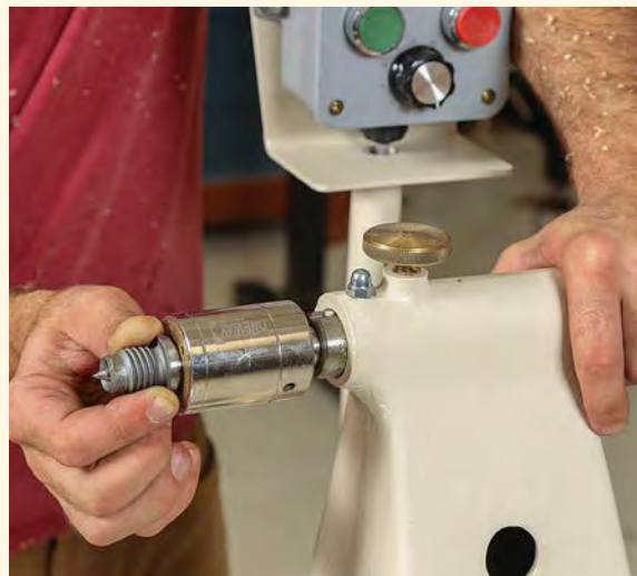
Live center. The Oneway's live center has an ergonomic design, is solidly built, and runs very accurately. A threaded, rotating, cup center can accept accessory centers.
