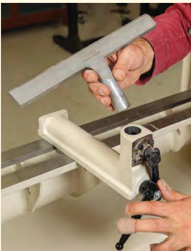
Prime parts. The Oneway's tool rest and banjo, like the Robust Scout's, are among the best commercially available.
