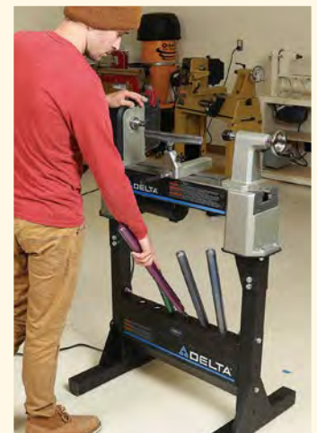
Give your tools a rest. The tool rest on the Delta is very easy to access to insert and remove your tools.
