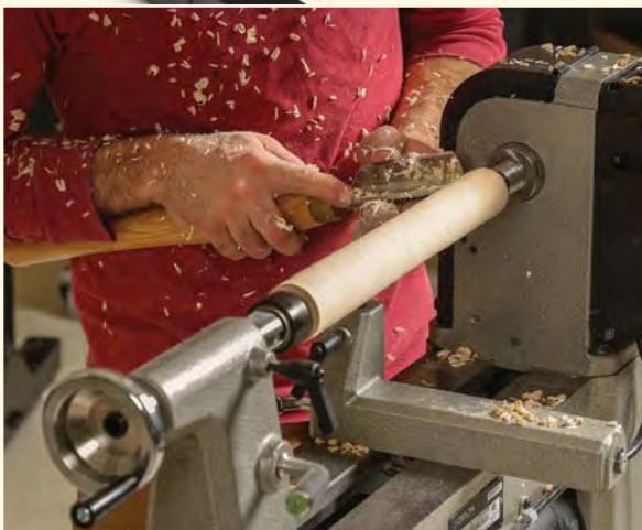
Streamlined design. The sparse design of the Delta allows the user a lot of maneuverability around it. Here Finnigan can rest against the machine to get right in line with the work.
