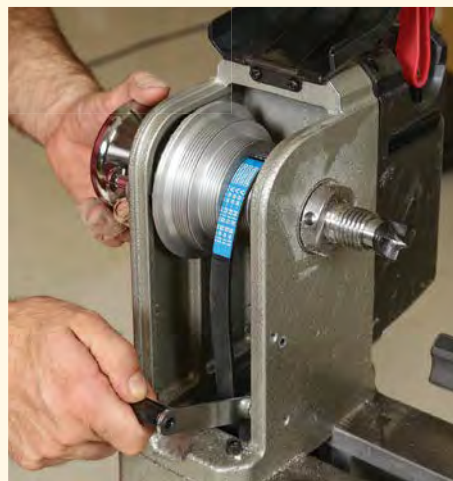
Speedy change. The controls were intuitive and changing belts was simple with the use of a side compartment and lever. Finnigan particularly liked the spindle lock design.
