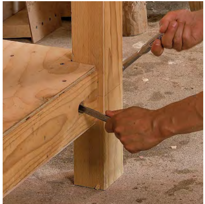
Shelf completes the base. Screwing in the shelf while the leg bolts are only gently tightened brings the sandbox stretchers into plane with the primary stretchers. With the shelf screwed down, Manney gives the bolts their final tightening.
