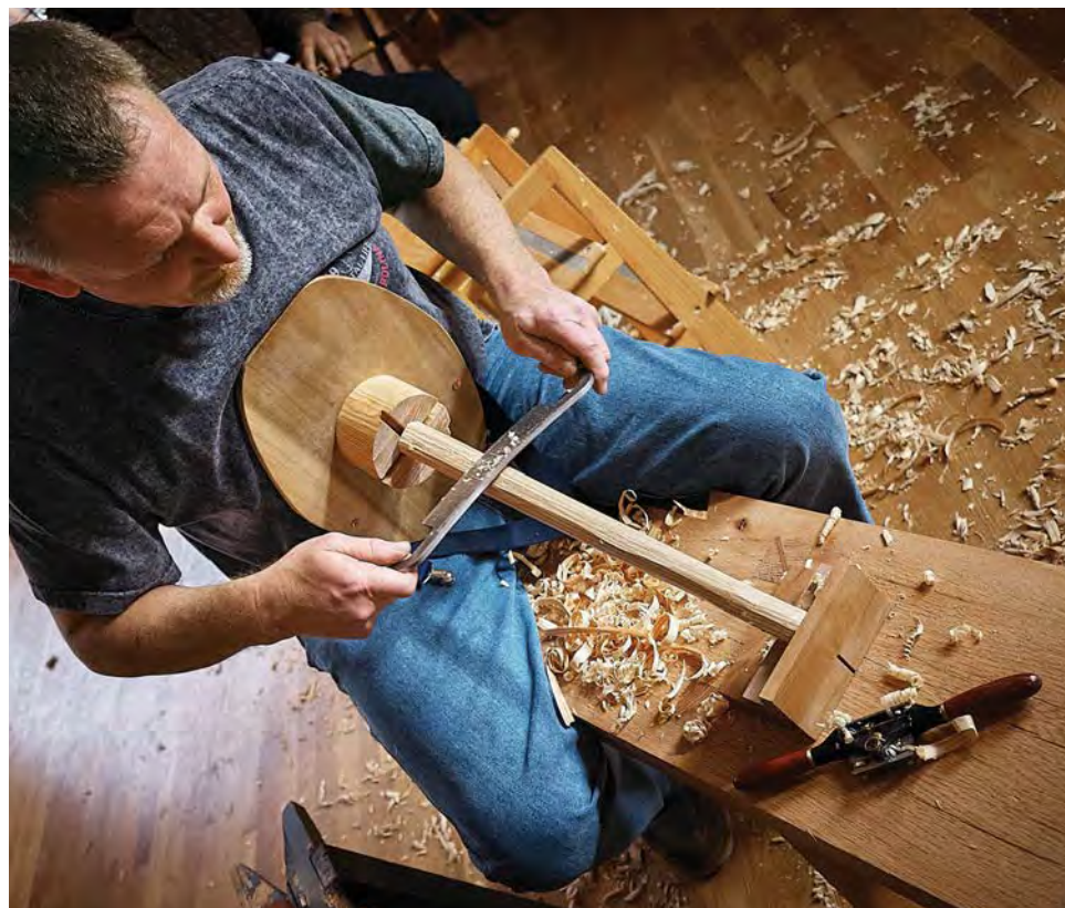
A head and a belly. Myers uses a “belly and head” to hold a spindle while he shapes it. With the circular plate resting against your belly, a chair leg or spindle can be wedged between it and a tiered block secured to the bench. Your body weight stabilizes the work while you shave it to shape.
