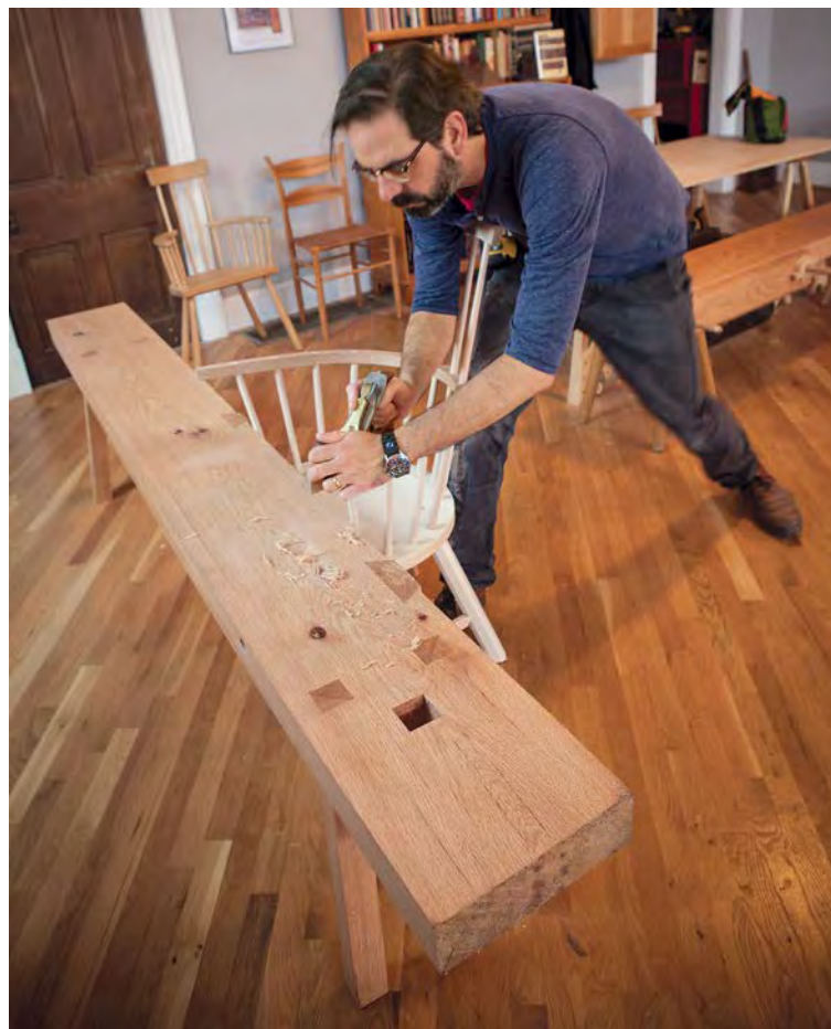
Traversing the board. It's easy to plane a board—especially a short one—on a low bench. Straddle the bench, with the front end of the piece against the bench pegs, and plane away.
