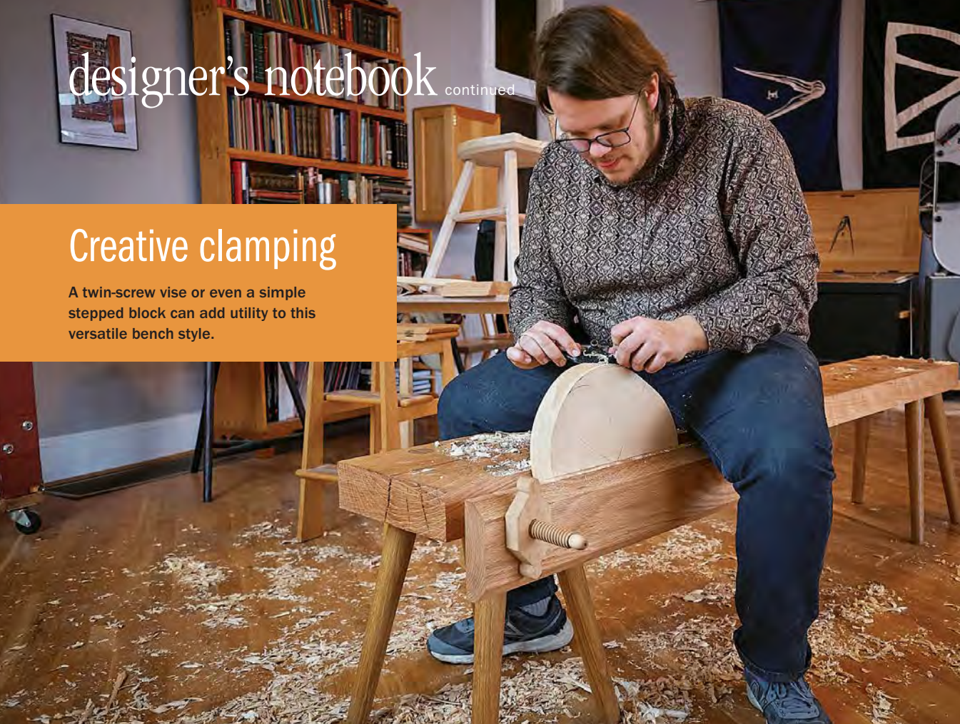
Screw vise. Brendan Bernhardt Gaffney uses a face vise, added to the side of the bench, to secure this chair seat while shaping.
