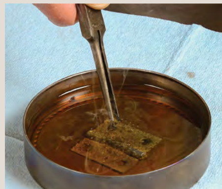
Add heat and quench. Using a blowtorch on a fireproof surface like this piece of granite, heat the hardware until you get a color you like. Use pliers to pick up the hot metal and dip it in linseed oil. Set it aside to dry.
