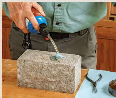
Add heat and quench. Using a blowtorch on a fireproof surface like this piece of granite, heat the hardware until you get a color you like. Use pliers to pick up the hot metal and dip it in linseed oil. Set it aside to dry.
