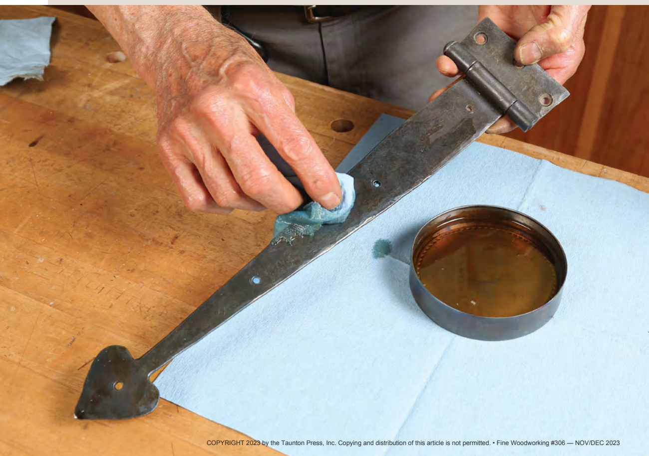
Just linseed oil. The bluish cast of wrought iron gets even more depth when you wipe on a coat of linseed oil.
