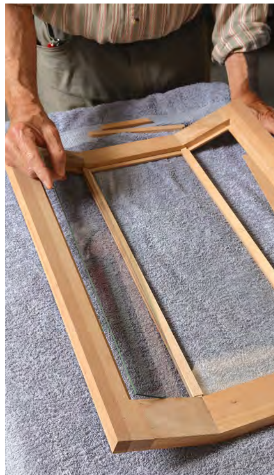
The middle pane of glass goes into place first. Slide the muntins onto the glass and lay the unit into the door frame, fitting the muntins to their notches. The outside panes slide first into the muntin groove on one side, then pivot into the stile rabbet.
