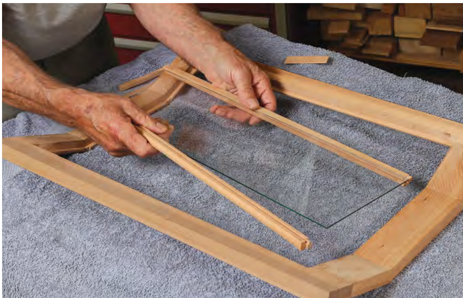
The middle pane of glass goes into place first. Slide the muntins onto the glass and lay the unit into the door frame, fitting the muntins to their notches. The outside panes slide first into the muntin groove on one side, then pivot into the stile rabbet.
