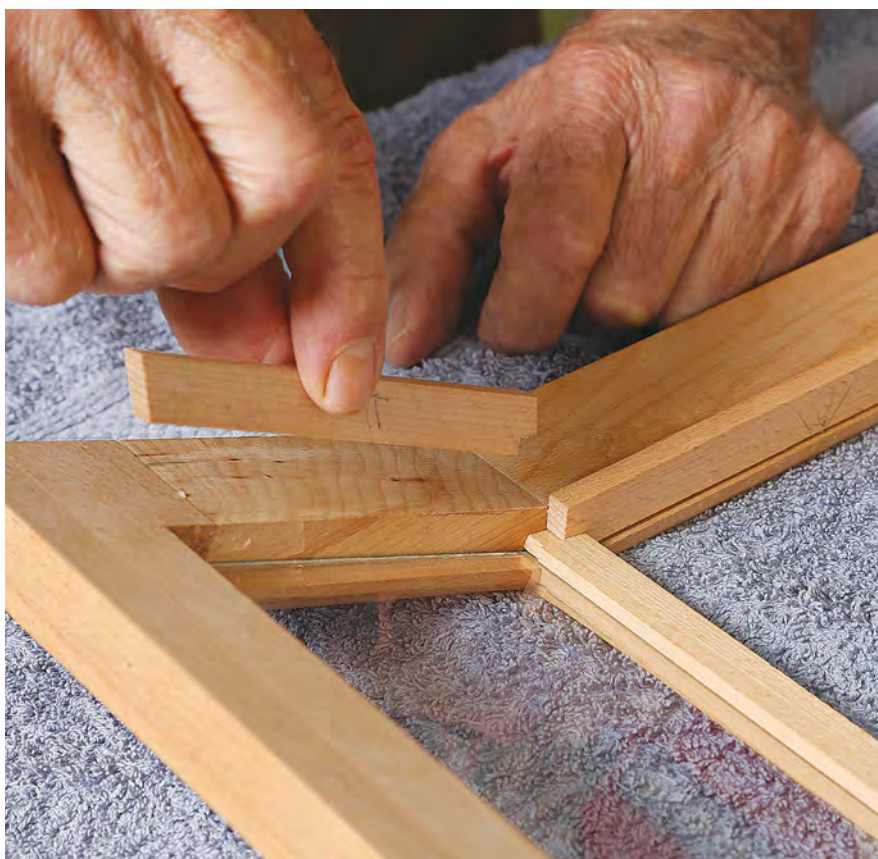
The middle pane of glass goes into place first. Slide the muntins onto the glass and lay the unit into the door frame, fitting the muntins to their notches. The outside panes slide first into the muntin groove on one side, then pivot into the stile rabbet.
