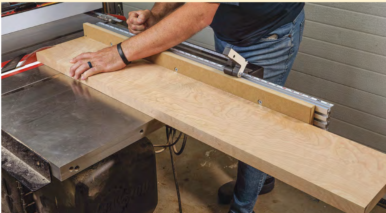
Large workpieces. This long, thick piece of hardwood represents some of the heavier stock a miter gauge might be asked to handle. Not all gauges were able to produce a perfectly square cut on this board, due to flex or play somewhere in the system.
