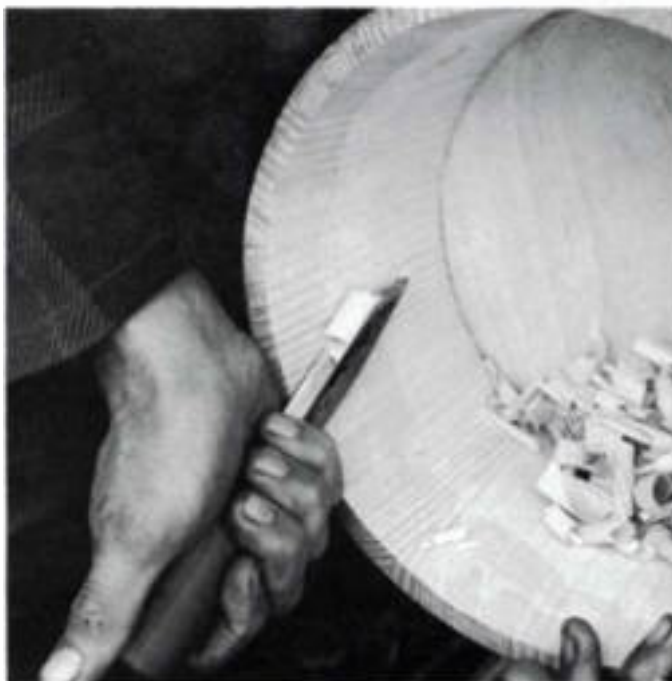
A knife sizes the rim line by beveling the waste away. Both the inside and the outside of the container will be thinned to meet these top and bottom rim lines.
