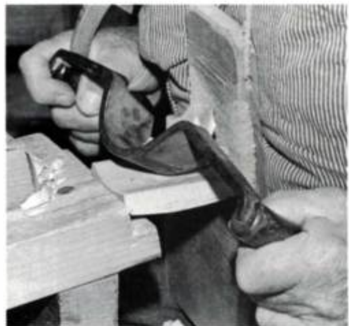
To shave short staves, cooper Ruedi Kohler supports one end of the blank in a rabbet on the front of his shaving-horse ledge, the other against a wooden bib.
