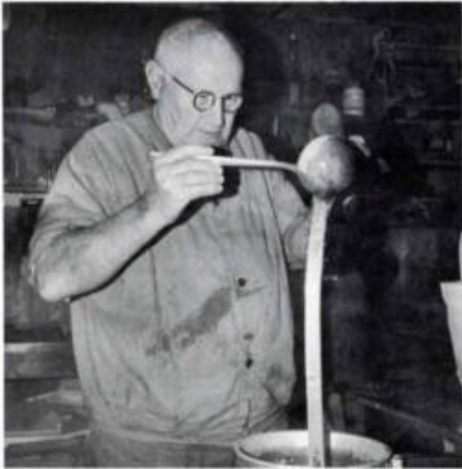
Ladling hot water over the hoop blank, above, limbers it for bending. The blank must be twisted, below, in order to fit one end through the other.
