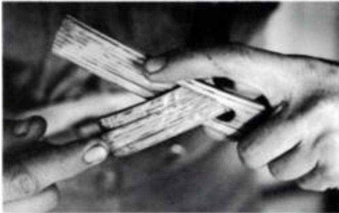
Ladling hot water over the hoop blank, above, limbers it for bending. The blank must be twisted, below, in order to fit one end through the other.
