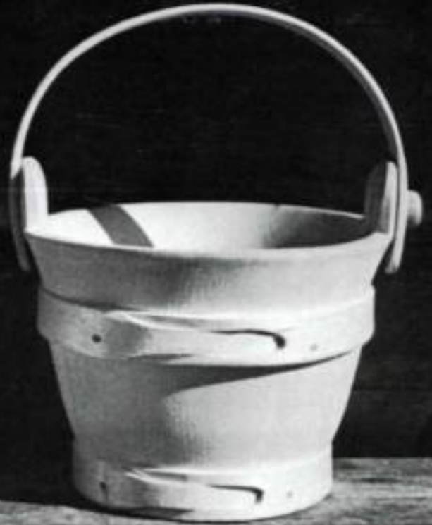
Swiss-style buckets of close-grained pine, with maple hoops. Traditionally used in small dairies, these liquid-tight containers are known as 'white' cooperage. The sculpted bucket, right, is carved from extra-thick staves after the staves have been glued together.
