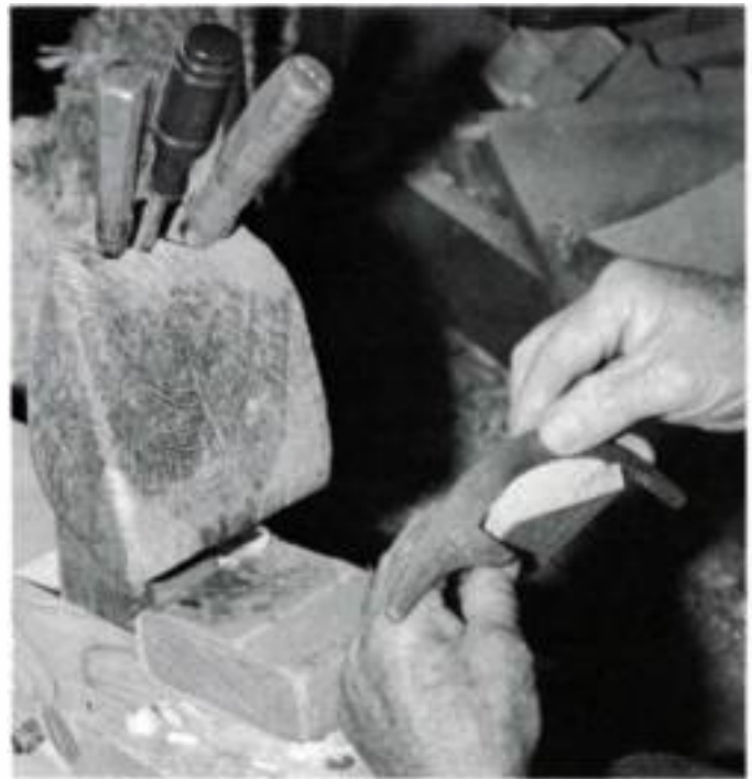
The outside curve and edge bevel of a bucket stave are checked with a gauge called a modell, drawn on facing page.
