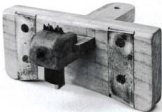
This croze is like a marking gauge with teeth. Instead of merely scribing the groove for the bottom, it cuts it directly into the assembled staves.
