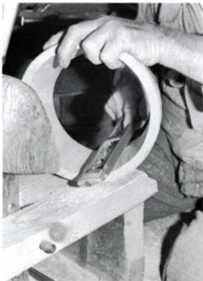
The staves are test-assembled and temporarily held in place with two metal hoops, so that the inside of the cylinder can be smoothed either with a convex-sole plane, as on the front cover, or with a Surform, above.
