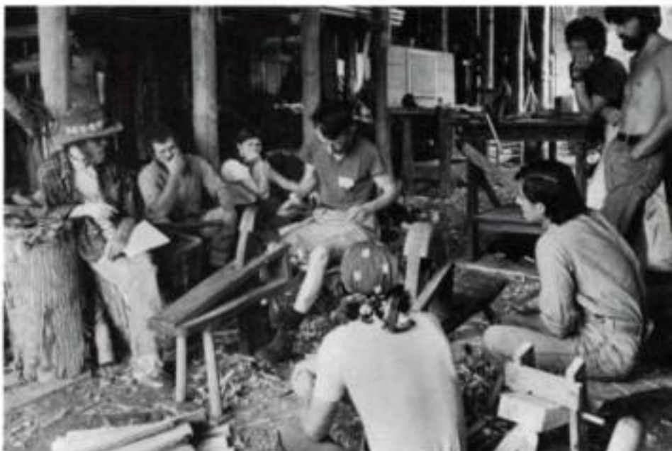
To make ten of Sawyer's chairs, left, one for each of us in the workshop, we started with a 6-ft. length of an 18-in. dia. white oak log. After quartering this with wedges to see the lay of the grain, we bucksawed lengths for chair parts. At top, two students saw a bolt for rungs. Steadying the log are Country Workshop sponsor Drew Langsner and his daughter Naomi. Above, teacher Dave Sawyer demonstrates drawknifing a rung on a dumbhead shaving horse.
