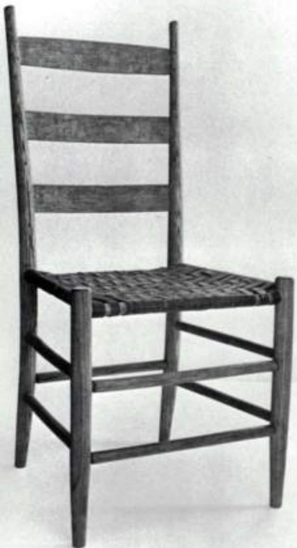
To make ten of Sawyer's chairs, left, one for each of us in the workshop, we started with a 6-ft. length of an 18-in. dia. white oak log. After quartering this with wedges to see the lay of the grain, we bucksawed lengths for chair parts. At top, two students saw a bolt for rungs. Steadying the log are Country Workshop sponsor Drew Langsner and his daughter Naomi. Above, teacher Dave Sawyer demonstrates drawknifing a rung on a dumbhead shaving horse.
