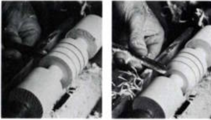
To start a ball shape, rub the bevel on the line, roll the gouge and lift the handle. Start each successive cut a little closer to the center line, but don't move the tool along the rest during any one cut.
