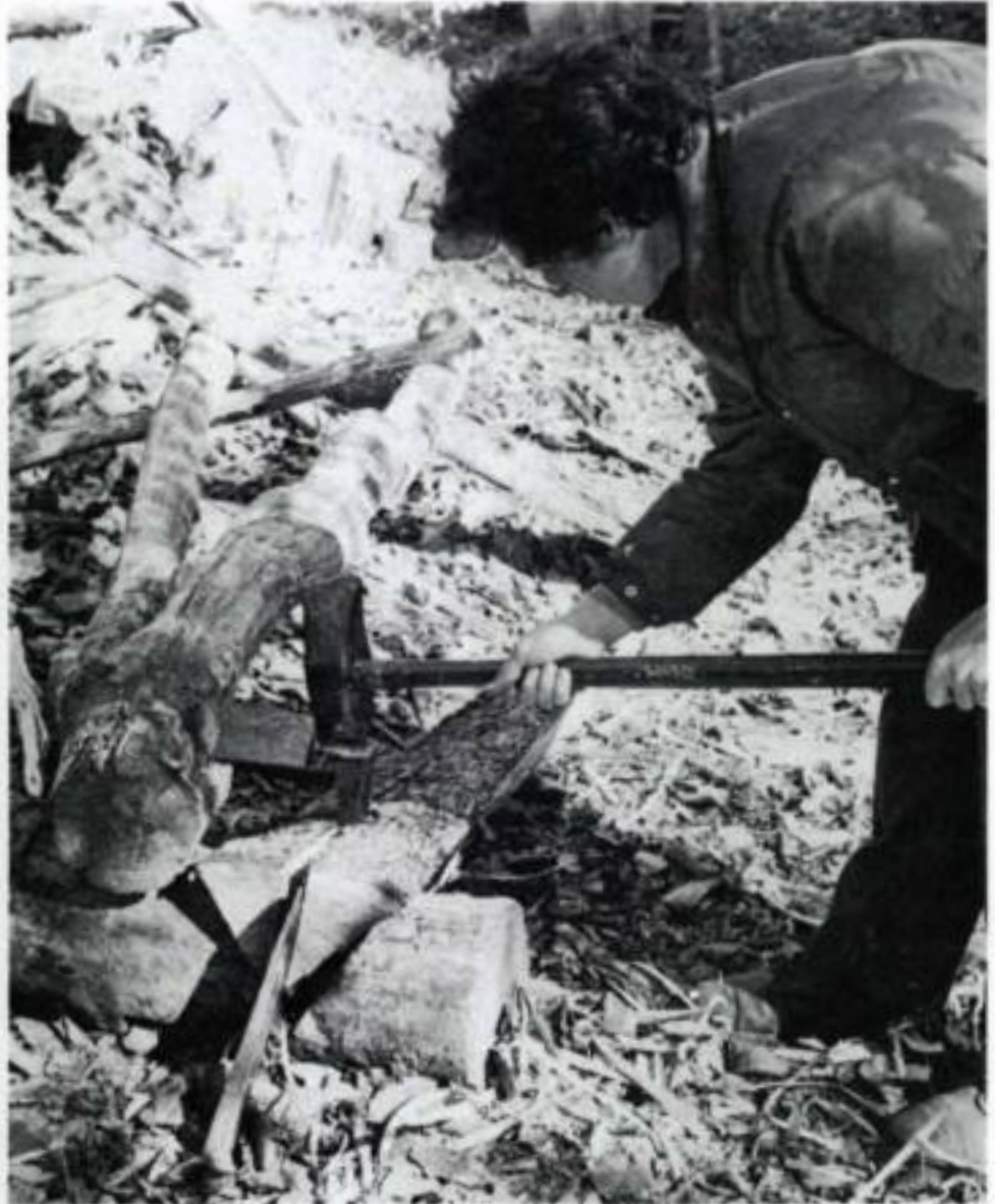
Hewing: With an iron wedge driven into the end of a white oak log (top left), wedges are leap-frogged along the cleft. Two 3-in. pluts and a dogwood cudgel complete the split (bottom left). Then quarters are cleaved into eighths with a pair of wedges and a 10-lb. go-devil (above). Note the splitting break at left, propped up by crossed saplings.
