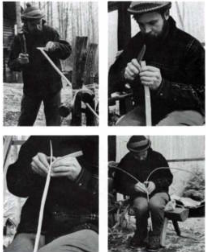
Top left: White oak stick supported by brake lashed to two posts is worked into basket splints. Then thin splints are held between the knees and further divided. A small knife opens the cleft (top right), then the pieces are pulled apart by inserting the thumbs into the cleft and sliding the fingers down the outside (bottom).
