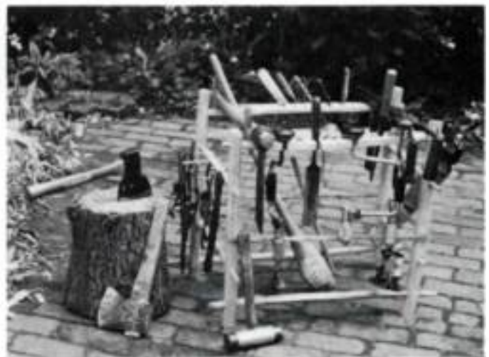
A post-and-rung tool rack can be made quickly from spare and rejected chair parts, bound together with a toggle rope.
