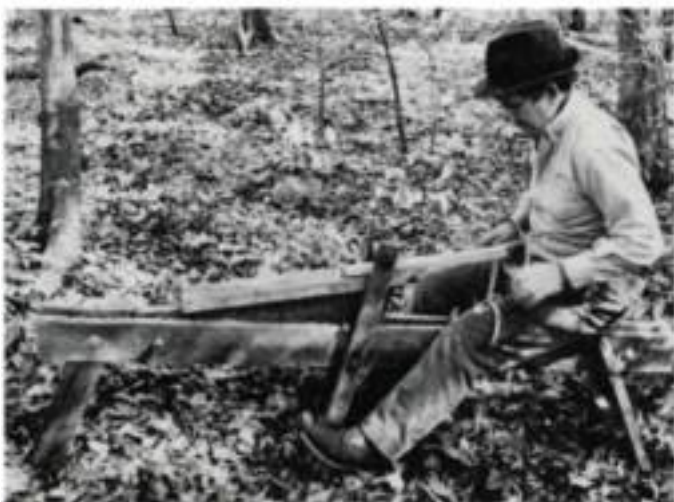
This style of shaving horse is light enough to be toted into the woods for drawknifing split sticks right where the tree is felled.
