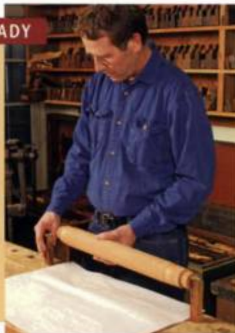
Cut the veneer to size. Make a paper template rather than bending the dry, brittle veneer. The veneer should overlap \frac{1}{2} in. at the seam.
