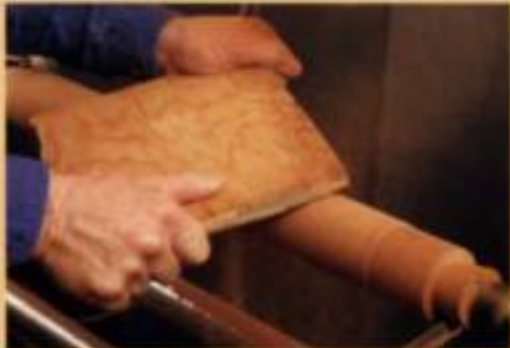
Turn a straight column and secure it well. Glue cloth-backed sandpaper to a square of plywood to make a low-tech smoother for turnings. To secure the column, make a set of extralong benchdogs (right), with a screw tip poking out of each. Also, tape off the tenon areas of the column.
