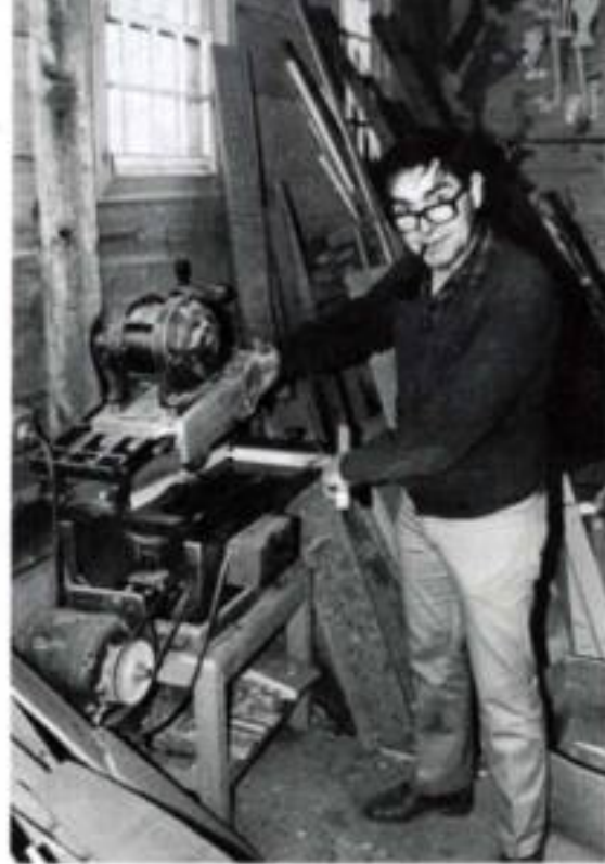
Left, Gerald Curry's reproduction of a Queen Anne highboy in walnut. Right, Douglas Campbell at his tenoner made from a Sears table saw. The extension table is hinged at the far end of the main table and is raised and lowered by a threaded rod. On this swinging table is mounted a 1-HP motor belted to a saw arbor. Both this arbor and the saw's regular one are fitted with plywood blades (to cut the tenon shoulders) and a Sears molding head with straight knives (to waste the wood and produce the cheeks). With a miter gauge and an angle block, Campbell's tenoner can quickly make the double-angled tenons on traditional chair stretchers.
