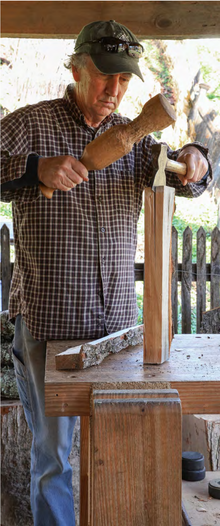
The bent blank starts out flat. Instead of searching in the woods for naturally bent spoon stock, as he used to do, Buchanan splits and shaves a chunk of green sugar maple and steam-bends it to create a curved blank.
