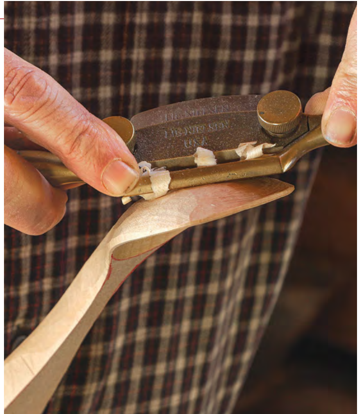
Spokeshave for fine smoothing. Having completed the majority of shaping with the drawknife, Buchanan follows up with a spokeshave set for a fine cut to smooth the convex surfaces.
