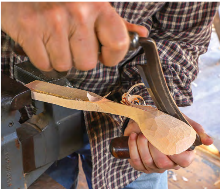
On to the handle. After rough shaping the handle with a drawknife, use a spokeshave to attain the finished form.
