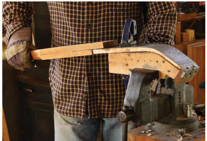
Bending form in the vise. A steel strap screwed to the bending form and bolted to a long wooden handle helps ensure successful bends. The blank remains on the form for two days.
