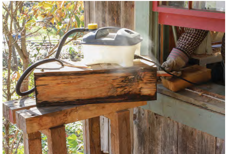
Steam bends the blank. After an hour in Buchanan's rough-and-ready steambox, the spoon blank is ready to bend.
