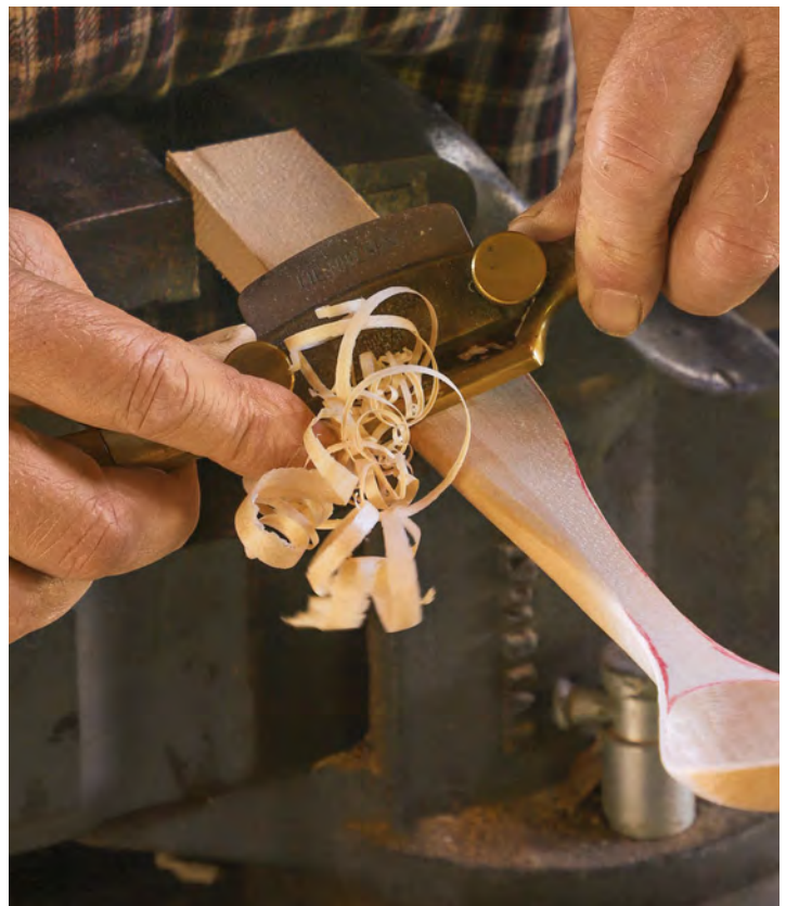
On to the handle. After rough shaping the handle with a drawknife, use a spokeshave to attain the finished form.
