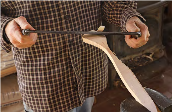
Beneath the bowl. Buchanan uses a drawknife to shape the back of the bowl, echoing its curve and bringing the rim to a narrow bevel.
