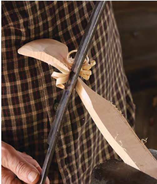
Beneath the bowl. Buchanan uses a drawknife to shape the back of the bowl, echoing its curve and bringing the rim to a narrow bevel.
