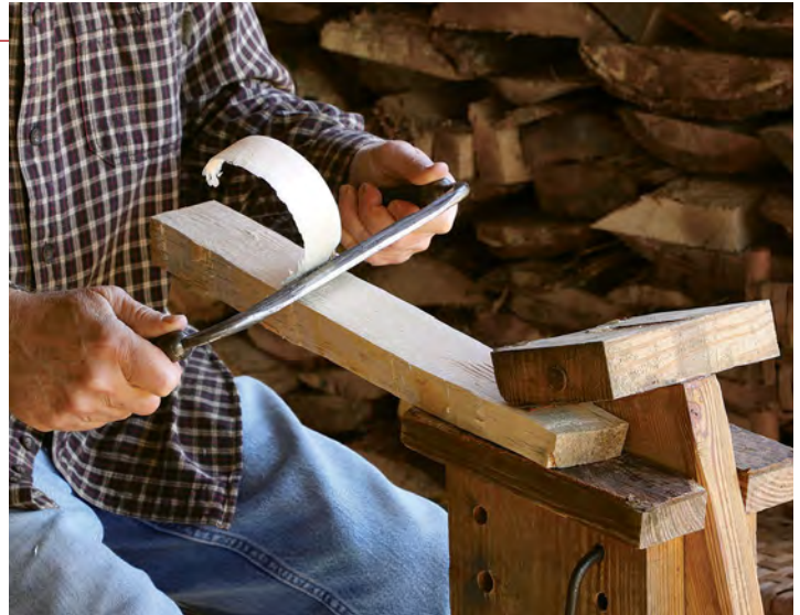
Drawing it down. Working the radial planes with a drawknife, Buchanan flattens both wide faces of the blank, bringing it down to a thickness of \frac{9}{16} in.
