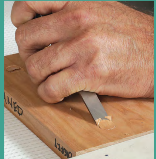
A sliver of each. Axelsen used a round punch and a chisel to create samples small enough to fit into the scanning electron microscope (SEM).
