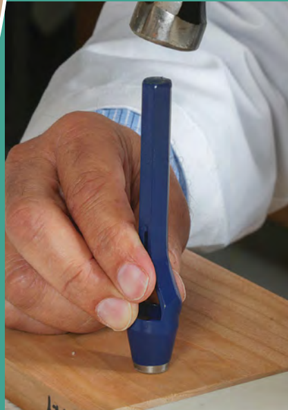
A sliver of each. Axelsen used a round punch and a chisel to create samples small enough to fit into the scanning electron microscope (SEM).
