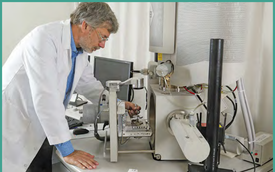
Into the scope. After applying an ultrathin metallic coating to each sample—required by the SEM—Axelsen loaded each into the microscope and examined its entire surface. He then chose the most representative area and best degree of magnification for each photograph.
