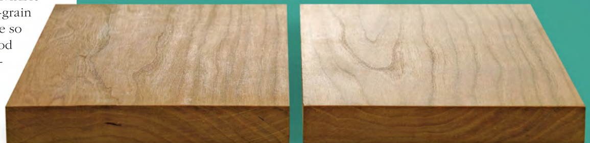
Reflected light tells the tale. Both of these cherry sample boards were given a single coat of boiled linseed oil. The board at left was sanded to 220 grit, and looks matte in reflected light. The sample at right was sanded to 800, and reflects the same light with a buttery sheen.
