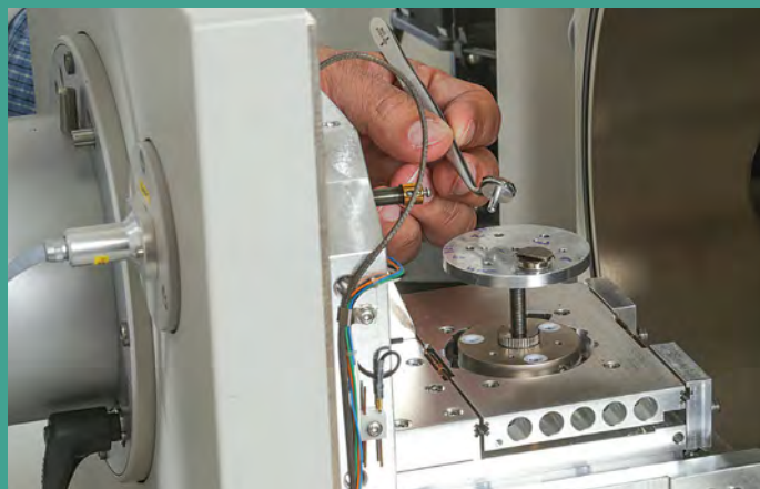
Into the scope. After applying an ultrathin metallic coating to each sample—required by the SEM—Axelsen loaded each into the microscope and examined its entire surface. He then chose the most representative area and best degree of magnification for each photograph.
